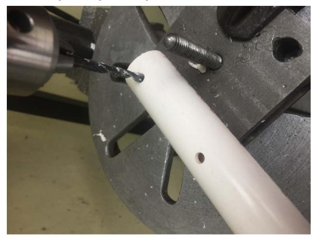
I set up a finger plate on my drill press and drilled one 3/16 inch hole near the end of the pipe and a second hole about 2 inches back.
