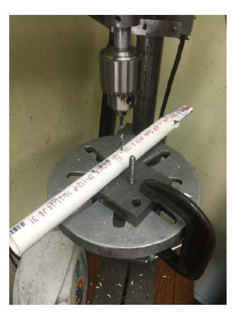
Back on the drill press, I cross drilled holes about every 2 inches.
