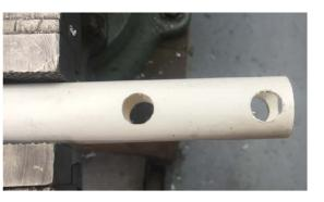
Then I enlarged the holes to ½ inch. The hole closest to the end helps guide the saw cuts.
