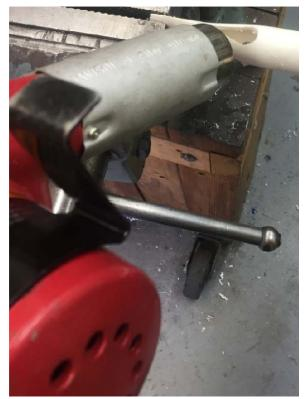
Using my heat gun, I warmed the PVC until it was very soft. Then I clamped the end of the pipe in my vise and sprayed the plastic with water to cool it.
