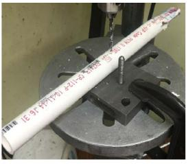
The stake is rough cut on my bandsaw and drilled by eye. The pointed end is heat formed using an air heat gun.
