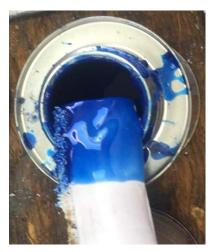
Then the end was dunked into PVC cement. I pried the ends open a second time to let the cement flow in. Then I wiped the outside with a rag to remove the excess cement.
