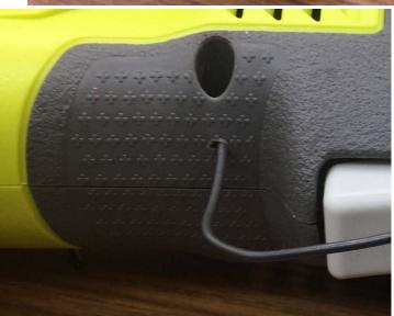
After removing the screw just below the trigger, I drilled an 1/8" hole tangent to the top of the chamber that held the screw. I then pushed the wire through the hole and formed a hook.
