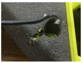
Next I notched out the rubber and plastic on the side of this hole. It was too shallow to drill a side hole plus the base of the compressor prevented me from drilling this hole at the needed angle.
