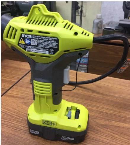
The first step was to figure out the best way to form up and anchor a trigger guard. I used some soft steel wire caught under existing screws.
