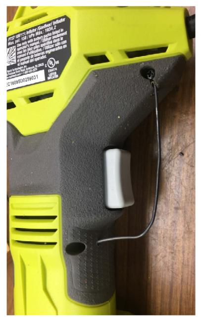
After installing the second screw, the soft wire guard was secure.
