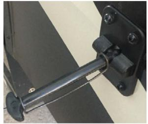
The existing anchor consists of a bar that swings out which is attached to the trailer wall and
