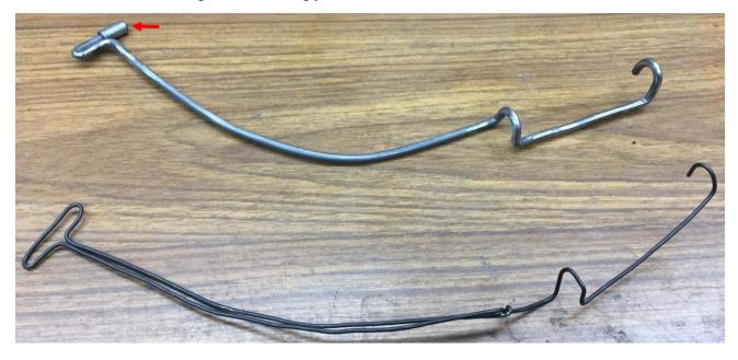
That sleeve on the end (red arrow) that fits into the receiver is a correction needed because I cut the wire about 1/8 inch too short.
