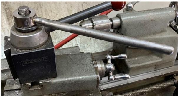
I didn't have the correct size box wrench to modify but did have a spare socket. Since the torque requirements were modest, I silver brazed a steel rod to the outside of the socket.
