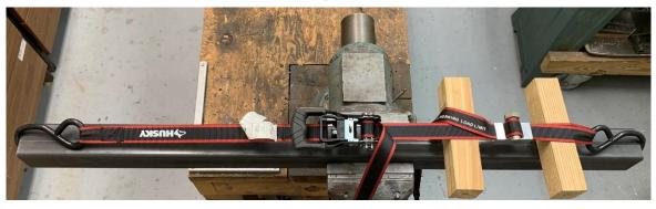
I don't own a scale able to read this tension but can operate the ratchet either until I or the buckle fail. Note that I used a piece of ½-inch diameter steel as my bar. I was testing the buckle and didn't want the bar to fail first.
