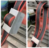
When done, release the tension and pull out the bar. The buckle falls off.
