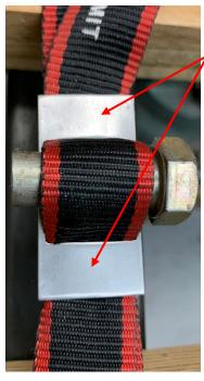
The bar is pushing on the edge of each flank while the flat part of the buckle is being lifted by the belt.
