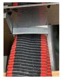
I could see that the top of the buckle crowned, and the flanks bent inward. My square, referencing one flank, tells the story.
