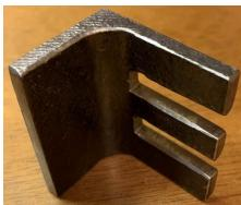
I then made a second buckle with ¼-inch thick steel angle. The finger side is 1¼-inches long, and the other side is 1-inch long. You can see the large fillet in the corner. It plus the non-finger side of the buckle do a good job of anchoring the fingers.
