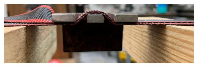
Here you see the new buckle in my test fixture. The belt is as tight as I can make it. The fingers do bend a little bit when the tension is removed, they return to their original position.
