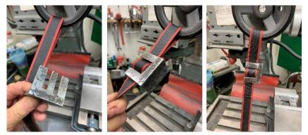
I ran my loop, slid on the clip, and applied tension. With the tension released, the heavy buckle remained in place. Yet I can easily lift it off of the strap by compressing the loop below the buckle.
