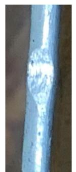
The round bar contacts the edges of the flanks in a small area. This concentrated the force and dented the aluminum. The flat bar distributes the force over a much larger area.
