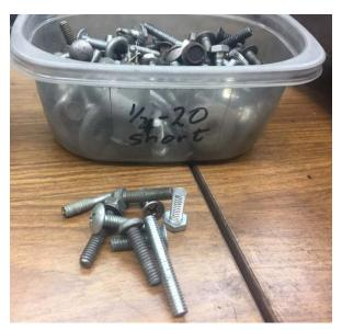
Next, all of the larger bolts were dumped into the tray. Out came the  $\frac{1}{4}$ -20 fasteners. Just remember to first match identical threads and then identify it.
