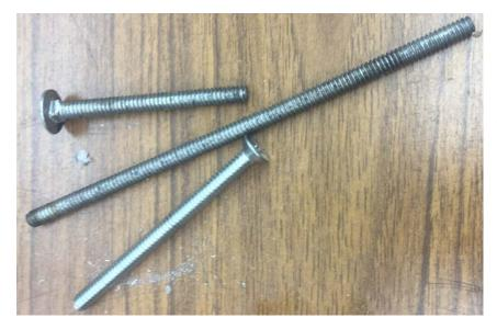
At this point, it was easy to match identical threads and then realize they were 10-24 bolts and rod.
