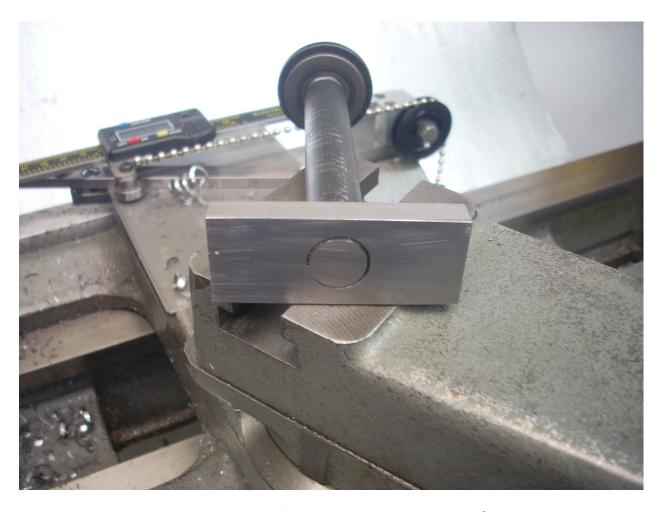
You can see that the bolt threads all the way to the bottom of the T nut.
