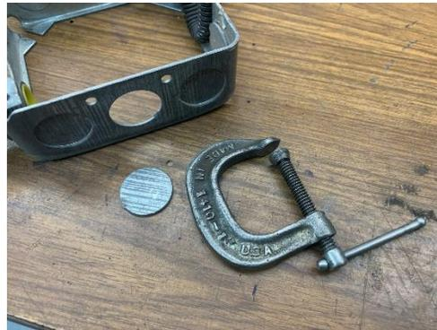
It doesn't matter if the anvil of the clamp is larger than the punchout since you are pushing into the box. Just be sure the foot is smaller.
