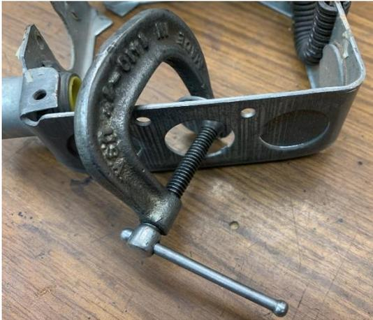
With all of this leverage, the punchout can be bent back and forth a few times and falls out.
