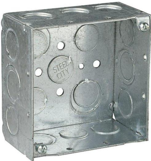
Most of the time, removing a punchout from an electrical box can be done with a hammer and a screwdriver. The single diameter holes break out easily. The ones with two diameters are more of a fight.
