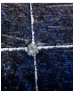
Push down on the punch, and you have a divot right at the intersection. The point of a small drill will drop into this divot. For larger drills, the divot can be enlarged with a bigger spring-loaded punch.
