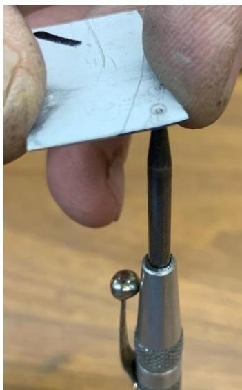
I then filed the bump off and verified that the point of the punch barely poked through.
