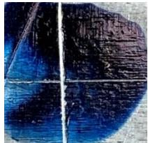
The standard way to accurately locate a drill on a flat piece of stock is to start with a dot of layout dye. Then a knife is used to scribe perpendicular lines. And finally, a layout punch is dragged along one line until you feel it go into the groove. Follow this groove until you feel it drop into the second line.
