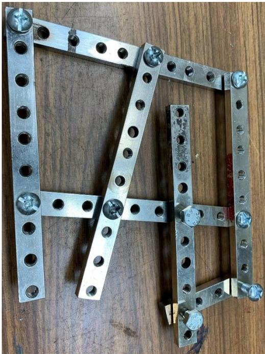
Ah yes, but what *good* are they? Mostly I use them to help me visualize parts of machines I wish to build. The value ranges from seeing how it moves to being able to build the machine. There are times when I use these bars as tooling, like the time I built a clamp for welding. See the partially ground off scorch marks?
