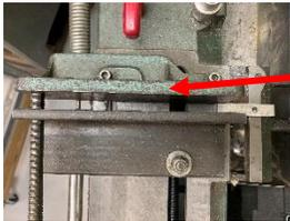
This procedure enables the user to adjust the fixed jaw on their horizontal bandsaw to make cuts that are as close as possible to square with the saw blade.
