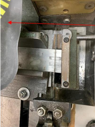
With the movable jaw pushing on the edge of the stock, I lowered the blade in preparation for cutting. I'm using my AirShim<sup>5</sup> to slow the downward feedrate. This is necessary in order to minimize both the burr on the bottom edge plus error due to excessive feed rate.
