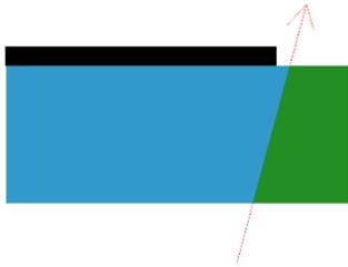
Say I have been blessed with a horizontal bandsaw that cuts a perfectly straight line with perfect repeatability. When the test stock is pressed up against the fixed jaw (black bar), I make this out-of-square cut with the blade (red arrow showing path and direction of cut).
