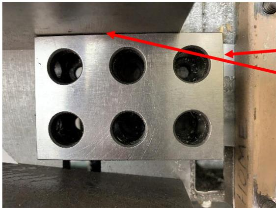
Here I have pressed the end of the 1-2-3 block against the cut edge while also pressing the loose fixed jaw against the flank of the block. You will have to imagine my fingers doing the pressing since they were busy operating the camera.
