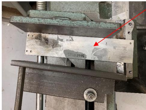
I placed a piece of scrap  $\frac{1}{8}$  inch thick, 2 inches wide stock against the fixed jaw.
