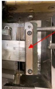
A length of  $\frac{1}{2}$  inch square tubing and two  $\frac{1}{4}$ -20 screws create an outboard clamp<sup>4</sup>.
