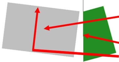
An object with a perfect right angle, like an ideal square or 1-2-3 block, can contact my reference surface and have a secondary reference surface that is perpendicular.
