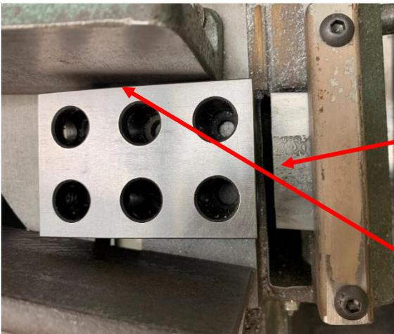
Even though the stock was way out of alignment, the saw cut will be aligned with the blade to within the repeatability of the saw and straightness of the cut.
