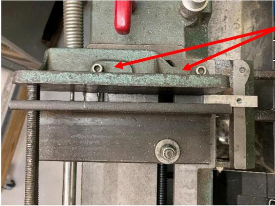
You could drill and ream two 1/8<sup>th</sup> inch diameter holes through the fixed jaw and underlying table. Then press dowels through the holes. This will provide very accurate alignment<sup>7</sup> if the fixed jaw must be moved and then put back. However, over time, the bandsaw will wear and it is possible that the position of the blade path will shift. This will cause the ideal position of the fixed jaw to move. Then one of these pins would be in the wrong position.
