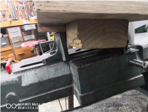
*The table is clamped in the vice on a bit of 2x4” screwed and glued to the under-side. It is tipped up the required amount with a piece of 18mm (near 3/4”) timber under the back edge that rests on the top of the moveable jaw. I didn’t shave any angle on the 2x4, it just clamps against the back edge ok. The plywood is 15mm thick, and the 20mm steel strip for the fence just screwed to the 15mm edge. The steel strip is almost cut through, so the plywood sheet is*
