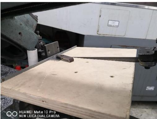
*I made a table out of plywood with the ~8-degree angle of the blade to table as proof it could work. I opted to put the table on top of the vice jaws so I could get the full 8+ " and made it wider on the outfeed side, so it is easier to clamp there.*
