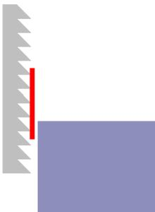
The way to limit how much metal each tooth removes is to have many teeth cutting at the same time. That is fine when the stock is thick enough, but
