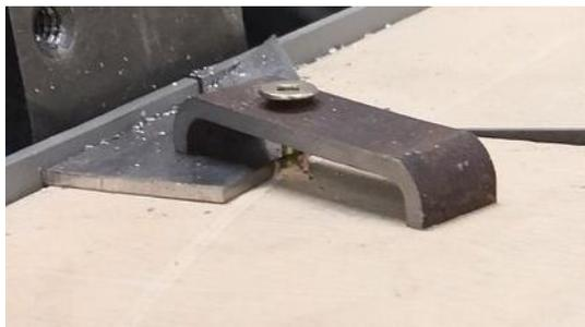
*What do you think of my little clamps? [RGS: Wonderful idea!] No need for a packing strip under them! They’re 5/8” wide, sawn off a 2 “x2” x1/8” with an oversize hole drilled ~1/3 of way along, so can reverse to get best fit to a predetermined hole pattern, but I just used wood screws straight into the ply. You’d*
