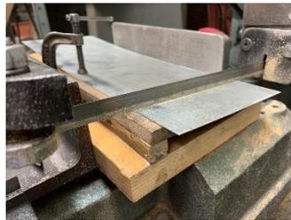
I drilled and tapped an array of  $\frac{1}{4}$ -20 holes on 1-inch centers. This lets me place my hold-down clamp where needed. The clamp steadies the sheet metal. My fence presses on the edge of the sheet metal to resist the cutting force. The holes to the right of the blade do come in handy if most of the stock is on that side.
