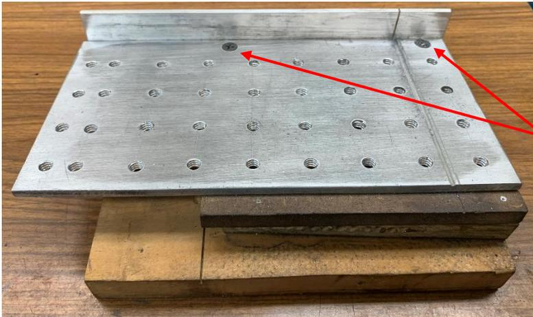
The force of cutting tends to push the plate into the fence and down on the tilted wooden platform. I, therefore, only needed two woodscrews to secure it. Be sure to countersink them, so the top of the heads is flush with the plate.
