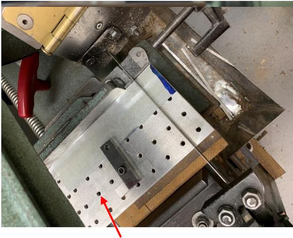
The plate is mounted to a board and set to an angle that approximately matches the angle of the blade. My goal was to have many teeth cutting at the same time. I did not try to select an angle that would have 3 or 4 teeth cutting at the same time, but that would have sped up the process.
