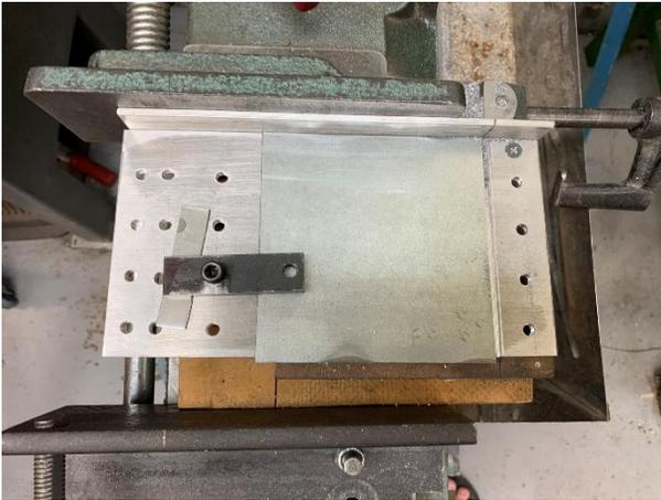
My fixture consists of an aluminum plate with a fence on one side.
