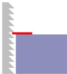
If your goal is to tear the teeth off of a bandsaw blade, quickly feeding sheet metal into a vertical bandsaw will likely get you there.
