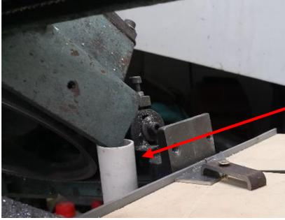
*See the bit of conduit ~4" long that slots over the sawframe stop to prevent the table being cut in half. Its doesn't work that well as it has to lean backward to capture the corner of the sawframe casting, but it's better than not having it.*
