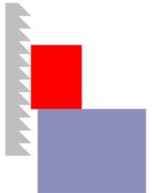
If you feed in very slowly, you can cut the sheet metal with no damage to the blade. The trick is to only remove a few thousandths of an inch of metal per tooth. Not so easy to ensure when hand feeding.
