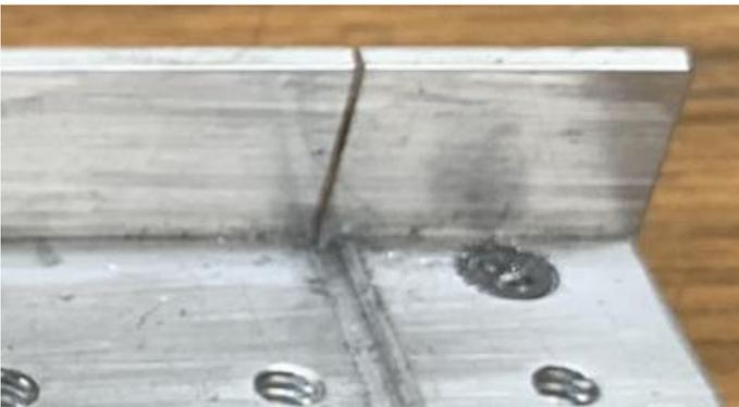
The most critical part of this attachment is the vertical cut in the fence. I align my scribe mark in the sheet metal to the left side of this cut when my scrap is to the right.
