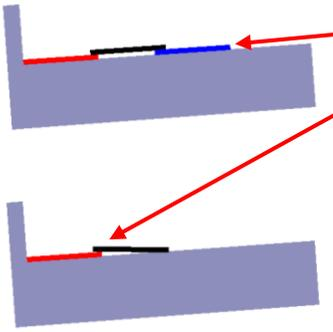
Notice a scrap of sheet metal under the hold-down clamp. This ensures that the clamp lays flat on the stock for maximum grip. Otherwise, the clamp would tilt and only press on an edge. Not the best clamping action.
