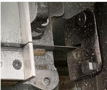
When installing the fixture, I loosely place it in the vise, lower the blade, and slide the fixture around until the blade enters the slot with no scraping on the sides. Then I tighten the vise. Alignment procedure complete.
