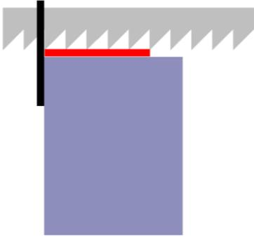
By changing to a horizontal bandsaw, we can have multiple teeth in contact with the surface at the same time. We just need to have a fixture. The black, vertical bar is a fence that stops the stock from being pushed off of the table. The fence has a slot in it to permit the blade to pass.
