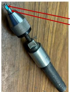
Next, I located a spare hex bit. After mounting it in my homemade pin vise, I used my belt sander to reduce the "fins," so the area
