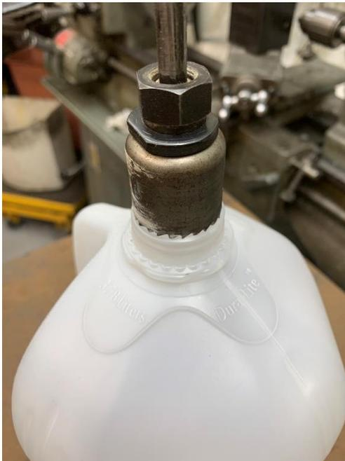
You will also need a 1-1/4 inch and a 1-1/2 inch diameter hole saw plus a drill.
