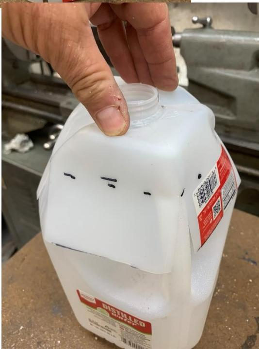
The top should drop over the the 1 gallon jug and provide substantial resistance when you reach the flange.
