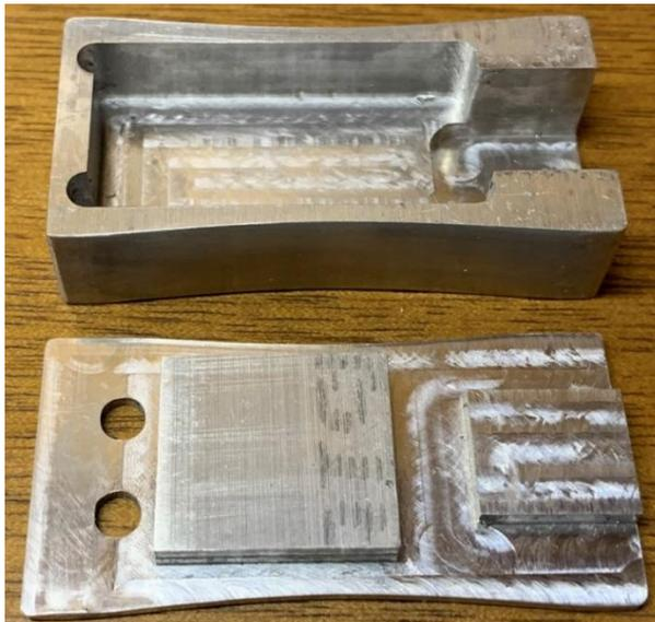
The bottom of the enclosure was CNC milled from a block of  $\frac{1}{2}$ " x 1" x 2" 6061-T6 aluminum.
