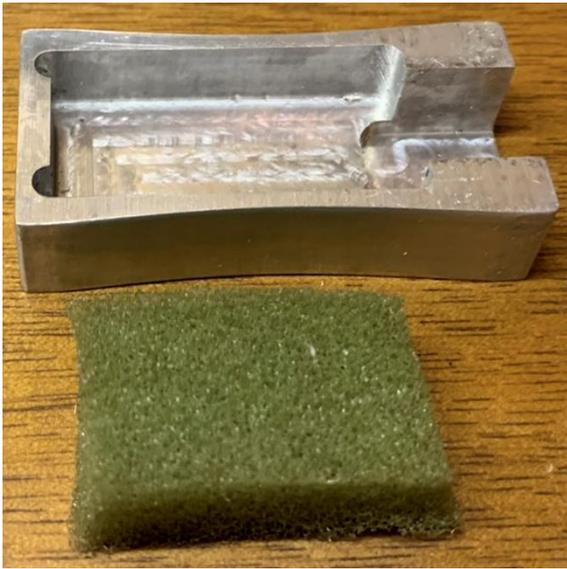
A rectangle of soft foam supports the circuit board.
