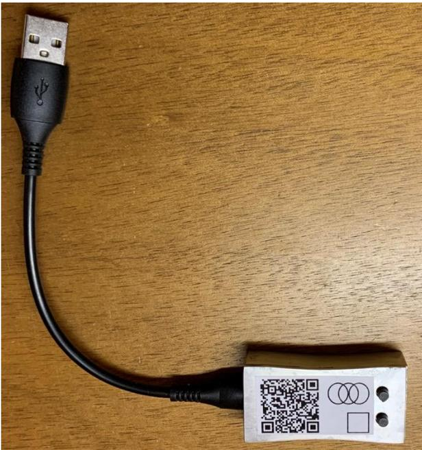
A detachable 6” long USB cable connects the device to the PC.
