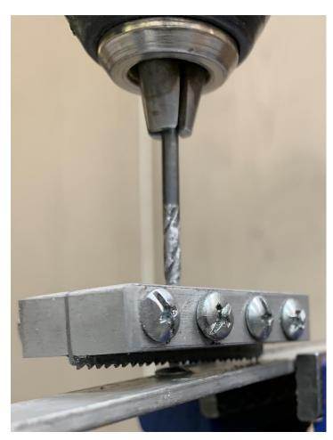
To use the tool, I slide my 1/8<sup>th</sup> inch drill bit through one of the holes. The teeth face towards the point of the drill.
