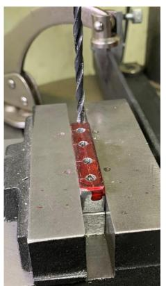
I placed the drilled block on the other block and aligned the ends. Then, I used the #36 drill to pass through the top block and drill the lower block. I had to be careful not to "tag" my vise ways on the end holes.
