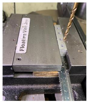
Again using the top block as a guide, I drilled matching holes in the bandsaw blade. The trick was to hold the blade down while clamping the block horizontally. I did this with my <u>holdown</u> <u>clamp</u> on the Floating Vise Jaw.
