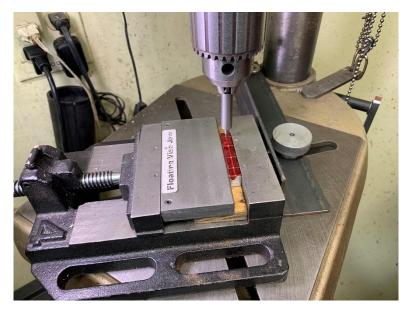
After laying out one of the bars for the four holes (two on the final design), I set up my drill press with a <u>fence</u> and located the first punch mark with my floating center drill cover<sup>3</sup>.
