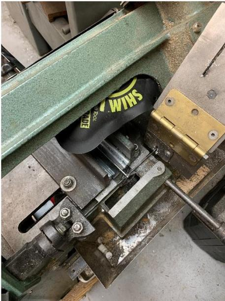
By using an “AirShim” which I bought at Home Depot for \$15 plus a small modification, I can limit the feedrate on my horizontal bandsaw. To see it in action, go to
