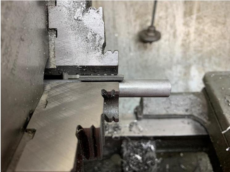
The stock is placed in my 3 jaw chuck with a 0.1" spacer between one jaw and the rod. This packing offsets the rod. The stickout is around 3/4 inch.
