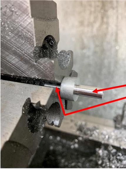
I needed to machine the second spigot so it aligned with the first spigot. Not a problem. Just held the part by the first spigot and took light cuts. If the 1/8 inch drill had not gone through this end, I would have spot drilled and drilled deep enough to get a through hole.
