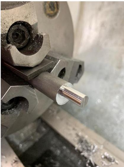
Most of the turning was interrupted cuts which slam into the cutter on every revolution. To reduce this jolt, I fed in only 0.01 inches per pass until most of the surface was being cut. Then I fed in 0.025 inches per pass. Machining stopped when the diameter of the spigot was about 0.01 inches larger than the inside diameter of the tubing I had chosen. Overall length was about 1/2 inch.
