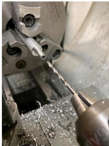
Next I spot drilled the end followed by drilling in about 1-1/4 inches with a 1/8 inch drill. Fed in about 1/8 inch at a time, retracted, and cleaned out the swarf embedded in the flutes of the drill. Used cutting fluid.
