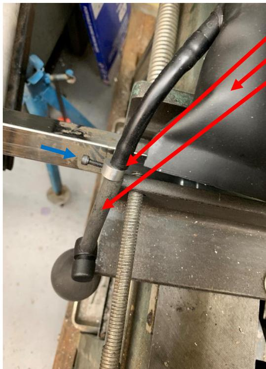
Here is the bleed valve installed between the Air Shim and new length of tubing. Gently tightening the screw (blue arrow) all the way down restores the Air Shim to normal operation. Backing it out just a little gave me the right amount of air bleed to lower my bandsaw blade at the desired rate.
