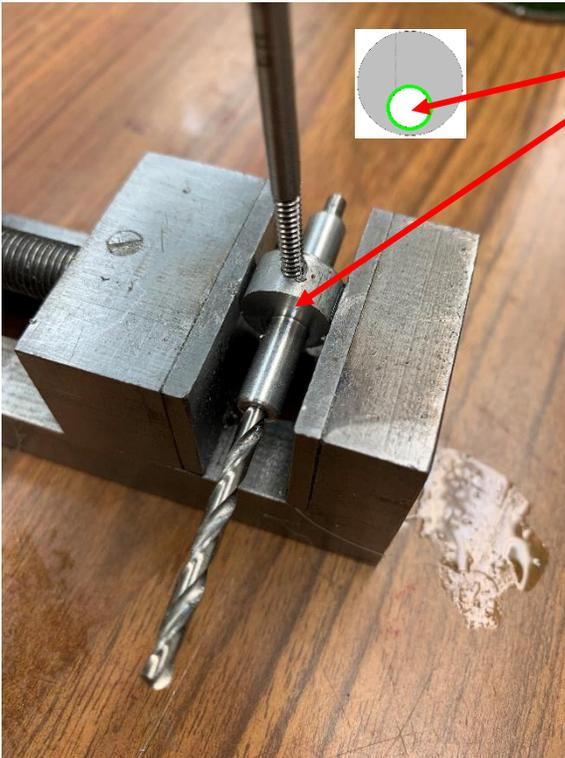
Moving over to my Drillpress, I first aligned the part in my vise so the spigots were at the bottom. This gives me the maximum amount of metal above the axial hole for tapping. I used a #36 drill to cut a hole down to the axial hole.
