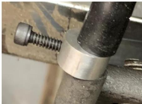
With this screw fully tight, the AirShim works normally and can lift up to 300 pounds and hold it there for a while. By backing out the screw, a small amount of air escapes causing a slow deflation of the AirShim. The bandsaw’s arm, resting on the AirShim, then descends at a controlled rate.
