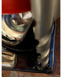
Then I selected a drill bit that is a close fit to the hole in the mounting plate. In my case, a 9/16-inch drill bit is a nice loose fit.
