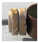
I positioned a pair of ball bearings inside wheels near the plasma cutter holder. These wheels are made from PVC because that was on hand. You can see the left wheel is already starting to melt. I will replace them with aluminum.
