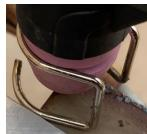
The guide is steel wire and clips on the ceramic nose cone. Note that the bottom of the guide does not form a circle.
