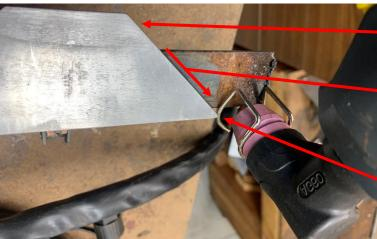
I would start with the torch off the stock with my guide providing alignment.
