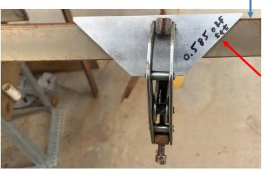
In this example, I clamped the angled guide to a piece of bed rail. This gives me a square cut on the face perpendicular to you (blue arrow) and an angled cut on the visible face. I'm thinking that the two cuts must align since I'm not moving the guide.
