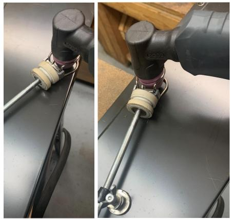
In practice, it was too awkward to constantly change the angle of the plasma cutter handle relative to me, monitor the coupler, and cut the arc.
