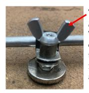
The wing nut made it easy to adjust the clamping force on the rod. Sadly, it tended to rotate and tighten as I pivoted my plasma torch. The rod would stop pivoting at some point, and the magnet would drag around as the torch moved. My fix was to use a locknut and let the screw pivot inside the magnet. I was able to adjust the clamping force so I could slide the rod as needed with no need of further adjustment.
