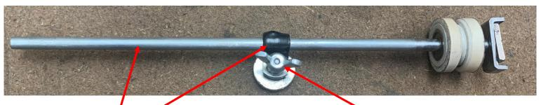
The <sup>1</sup>/<sub>4</sub>-inch rod, clamp, and wheels worked well. The wing nut and plasma torch coupler did not. This coupler consists of a bar magnet with a hole in the center and a U-shaped piece of steel. A 6-32 flat head screw secures the magnet and U to the rod.
