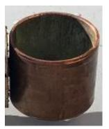
The plasma cutter holder is 1-inch ID copper pipe, 1-inch long. The top edge has been rolled inward slightly to catch the plasma cutter shield, while the bottom edge is smooth. The wheels should prevent this edge from contacting the surface, but it might happen, and I don't want it to catch. A flat head 6-32 screw secures the pipe to the end of the 1/4-inch rod.
