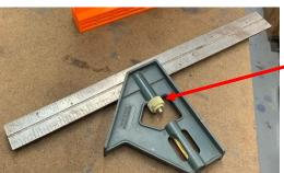
My lowly combination square gives me a generous edge at  $90^{\circ}$  or  $45^{\circ}$ . Furthermore, I can loosen the clamp and slide the blade as needed.
