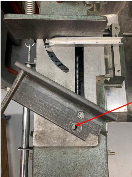
My movable jaw is free to pivot a lot more than necessary. As I crank it in, I have to periodically stop and move the left end closer to the fixed jaw.
