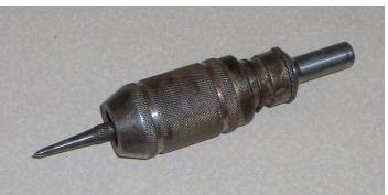
The shank goes into a handheld electric drill. With the drill running, John grinds the point of the punch to a uniform taper.
