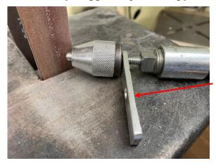
By holding the handle, I can spin the chuck without having it move sideways. Thanks, Marv! My pin vise just got a bit more precise.
