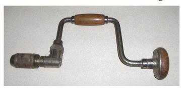
A brace and bit is designed to hold square shank bits.
