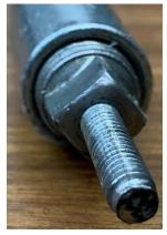
I drilled and tapped the plug \(^1/4\)-20 and screwed in a bolt from the inside. Assembly took no time at all.
