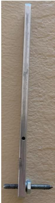
My tool is no more than a 1/8 - inch x 1/2 - inch x 5 - inch aluminum bar. I drilled and tapped one end 6-32. Then I took a 1-inch long piece of threaded rod and turned a point on one end. Screwed the rod into the bar and lock it in place with a lock washer and nut. Note that the washer and nut are on the same side as the point.
