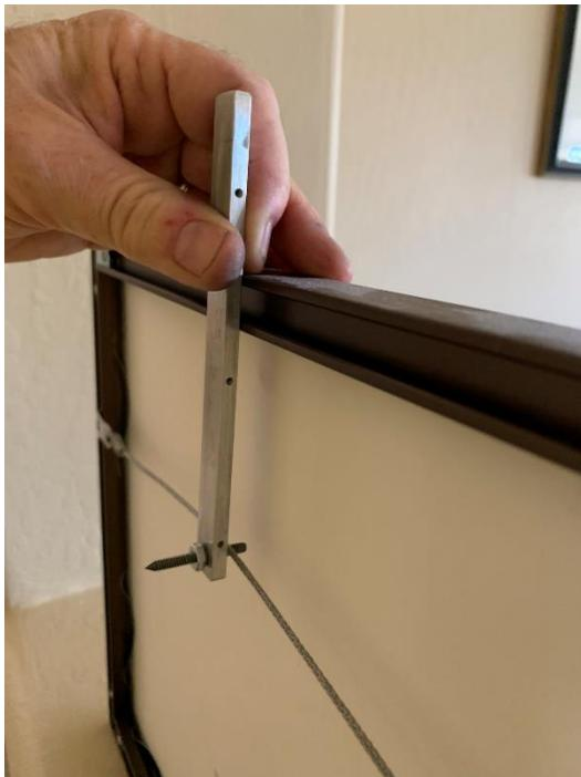
If the picture is supported by a wire, hook the blunt end of the threaded rod under the center of the wire, lift up, flip the picture over, and again use the bar to snugly push the point into the wall. Lift the picture away and push the point in deep enough to leave a mark.
