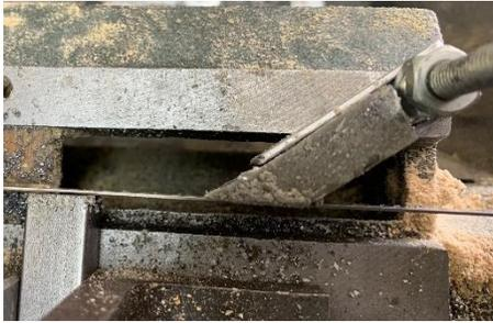
The table was drilled and tapped to accept the bolt. This hole can also be used as an anchor point for an outboard hold down clamp.
