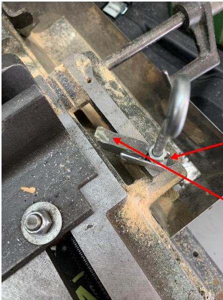
I have a small piece of aluminum channel that bolts to the table of my horizontal/vertical bandsaw.
