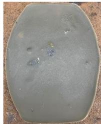
When cooled, the ingot drops out of the tub. I then use a knife to cut out a chunk.
