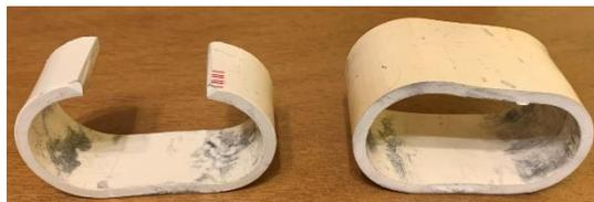
The clips were made from 2-inch diameter PVC pipe. Each one is about 1-inch wide.
