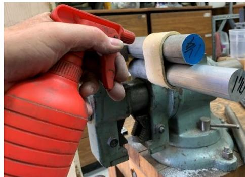
Spraying the plastic with water quickly hardens it. I repeated the process with the other piece of PVC.
