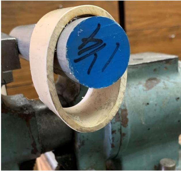
I started by sawing off two 1-inch lengths of 2-inch PVC pipe. The shaft of my paddle is 1 1/4-inches in diameter. With a round bar clamped in my vise and one of the pieces of PVC looped over it,
