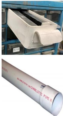
Four-inch diameter sewer pipe cost me ten cents an inch at my local Ace Hardware. With my heat gun and some scraps of wood, I turn this pipe into containers. Clear PVC cement lets me weld on bottoms and handles.
