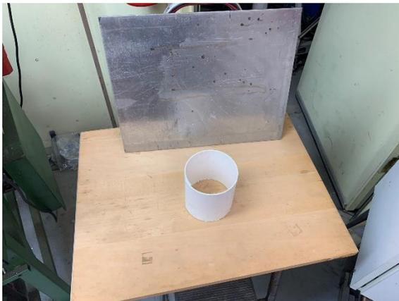
In preparation for making a PVC board, I have ready a flat piece of wood. The picture also shows a metal plate, but this turned out to be a problem. The metal cools the plastic too quickly. I later found that a second piece of wood worked much better.
