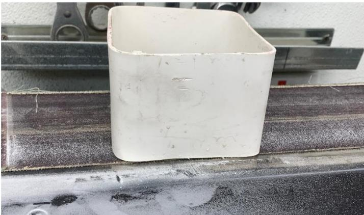
The top and bottom of the plastic box are slightly distorted. I use a light touch on my belt sander to true them up. The PVC cement can only work when the surfaces are in direct contact.
