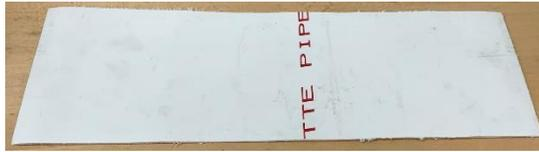
I quickly place the hot plastic on the board and flatten it with a second board. After about 30 seconds of pushing down, I end up with a nice piece of PVC board. Thanks to Nelson Collar for showing me this trick.
