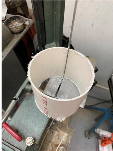
I then saw through the wall of the pipe.
