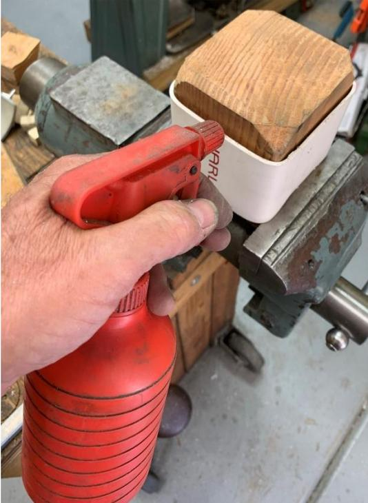
A bit of water sprayed on the plastic quickly makes it solid again. I can then pull the plastic off of the form.
