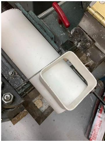
This box will have a floor, so I cut a second piece of pipe about 0.2-inches longer than the outside of the finished box.
