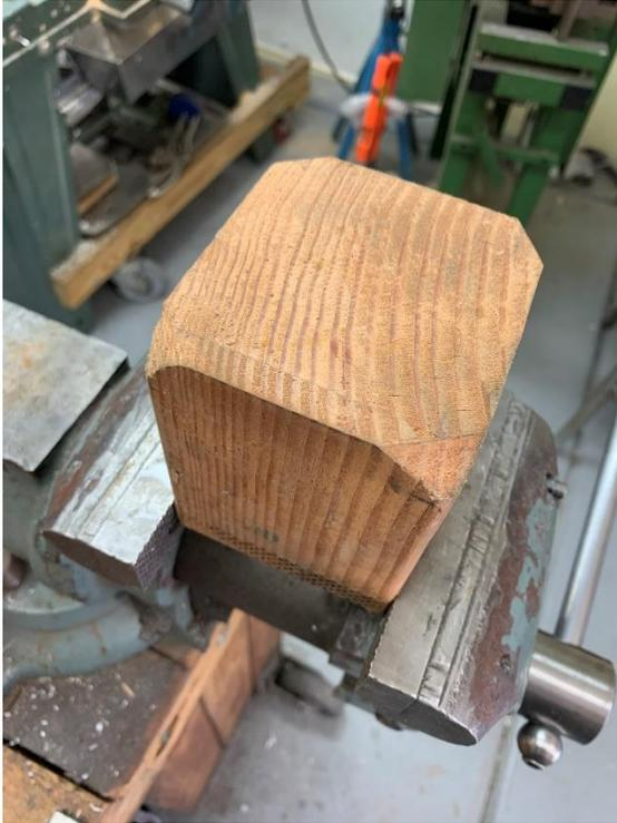
Purely by dumb luck, my box form is just a piece of 4 by 4. I beveled the top corners to make it easier to force on the hot pipe.
