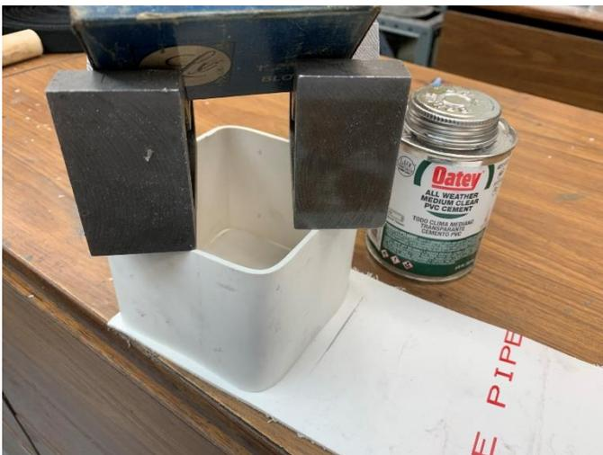
I coat the bottom edge of the box and the matching surface on my PVC board with clear PVC cement. After adjusting the parts to have a small lip on three sides, I put on some weights. Since I'm not in a hurry, I let it set up for an hour.
