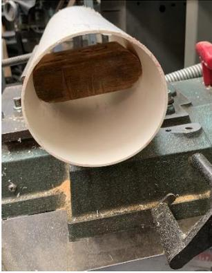
I first saw off a length of sewer pipe equal to the finished height of the box plus about 0.1-inches. In conjunction with the vise jaws on my horizontal bandsaw, the block of wood inside the pipe provides a solid clamping force.
