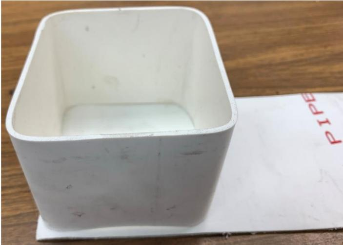
Even though there is very little contact surface, the box and bottom are securely welded together. Small gaps do exist, and this box does not hold water. If you want it to be water-tight, I suggest applying more pressure.
