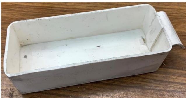
This box replaces a drawer. Again, by dumb luck, the correct size happened to have an inside perimeter of 14-inches. I later cemented on the pull and the stop.
