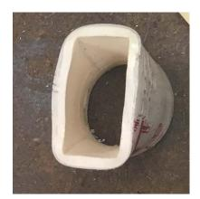
In this case I first blew hot air down the short length of pipe until it was leathery. Then I inserted two rectangular cross section bars and prying them apart for about 30 seconds. The result is a rectangular to round transition piece.
