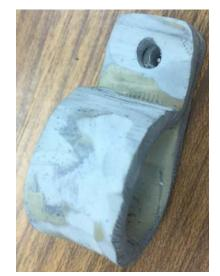
I rounded the corners and drilled the mounting hole. It looked very good. Then I tried cleaning up the surface with my 3M wheel and learned not to do that again.
