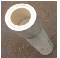
My first experiment was with a 5" length of 1" OD pipe. I held it in my lathe and ran at 26 RPM to insure uniform exposure to the heat. While I heated the end, I tested for the point where the plastic went from hard to a leather consistency. It is not an abrupt change and there is about 30 seconds of work time.
