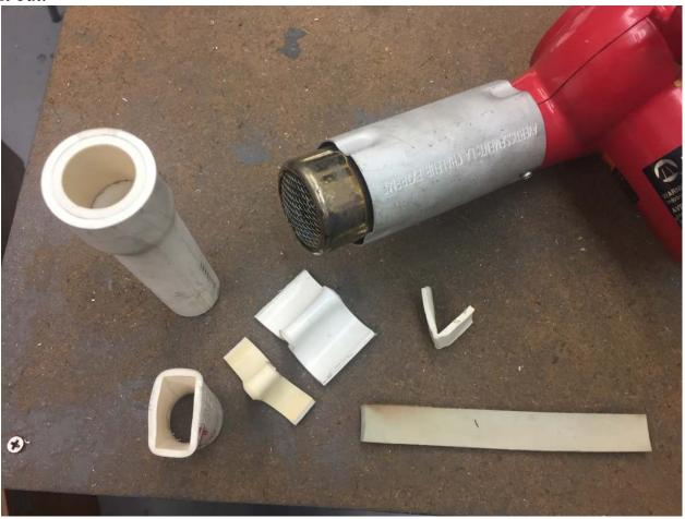
In all cases I used the commercial grade heat gun shown here. I think using a torch would be unsafe and also give poor results.
