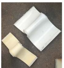
These two samples were created by first sawing through one side of a each short pipe axially. Then I heated the opposite side and pried them apart mostly with my fingers.
