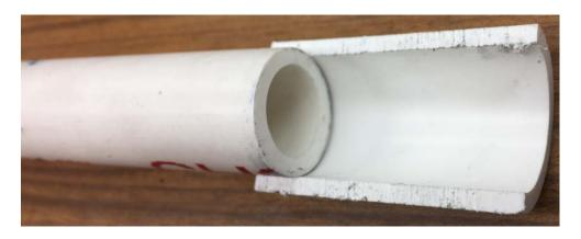
The patch's inside radius is a little bit smaller than the OD of the ½" pipe. Fortunately, plastic bends and the PVC cement sets up quickly.
