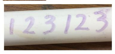
My first trial created markings that are a bit lighter than the full strength primer. As the acetone in the pen is driven out, the color will darken.
