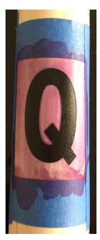
The technique involves masking off some of the pipe with stick on vinyl letters and 3M painter's tape and then applying PVC primer. When the primer dries, lift off the letters and pull up the tape. The primer does not appear to attack the vinyl so the letter can be reused.
