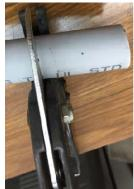
I used ABS plastic electrical conduit because it resists UV. It will see a lot of Arizona sun. Using a plastic pipe sniper, I cut off a 2 inch length.
