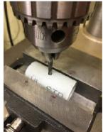
Then I cross drilled to make a clearance hole for the self tapping screw.
