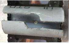
Looks a bit rough but fine for proof of concept. A deburring tool gives a nice bevel to the edges.
