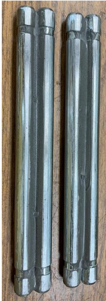
A pair of rods were placed on a flat surface and boxed in so they stayed in contact. Then I mixed up a batch of J-B Weld and formed a fillet between the rods. Once cured, I put each OO block on my belt sander to cut a flat on the epoxy side. This gave each block more contact area with the vise jaws.
