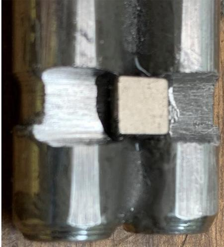
The final step was to enlarge the grooves in each end to accept a 1/16 x 1/8 x 1/8 inch neodymium magnet. This holds the block in place during set up. Had I realized the need for this recess before gluing, I would have cut them on my lathe.
