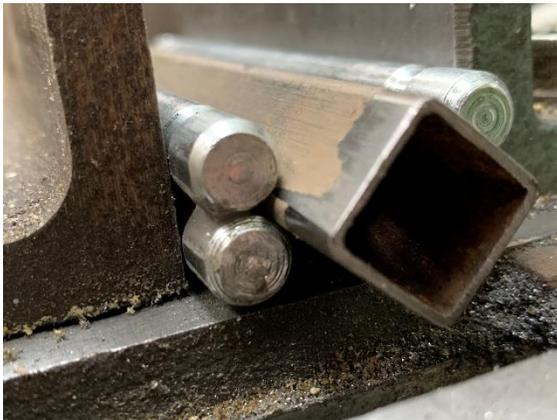
I’m using a pair of OO blocks to secure some square tubing as I prepare to cut it on my horizontal bandsaw. This has previously been done with V blocks but they take up a lot more of the vise’s capacity. The V blocks are also a lot narrower so the stock is not as well supported.
