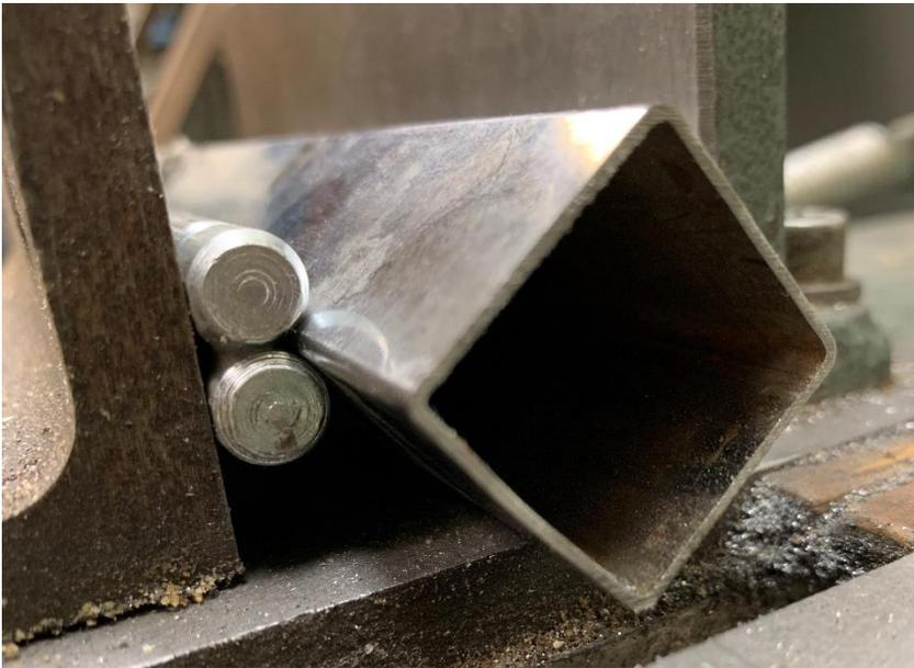
Here you can see a larger<sup>2</sup> piece of square tubing being supported by the OO blocks. The bottom corner is on the vise ways but the OO blocks are above the ways. I saw no rotation of the stock during sawing.
