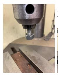
I threaded a short length of 3/8-16 rod onto a nut and chucked it into my drill press.
