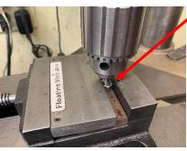
Then I lowered it into my vise and locked the jaws. Next, I locked down the vise to the drill press table.
