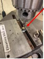
• I unscrewed the rod, screwed in a shorter length, and fitted my chuck with a spotting drill.
