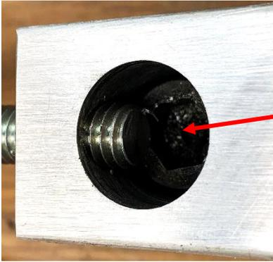
The positioning of the hole that passes the threaded rod takes some care. It must be high enough to clear the socket head cap screws that secures the aluminum block to its jaw carrier.
