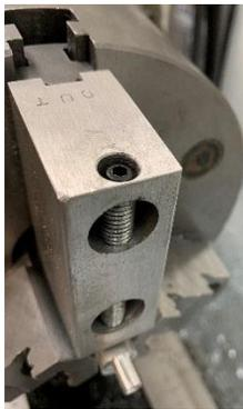
Here you see the custom jaw holding some 1/2 inch diameter aluminum round stock. Cutting the eccentric spud shown here felt the same as when I cut a similar part using packing.
