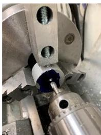
The clamping action occurs in the normal way: The chuck key is turned and all three jaws move inward until the stock is secure.
