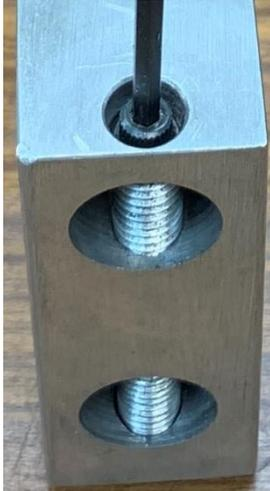
Note that when the square end of the threaded rod is flush with the bottom of the aluminum block, the screw at the top is flush. This is for safety. I did not want anything sticking out of the jaw that could hit machine or me.
