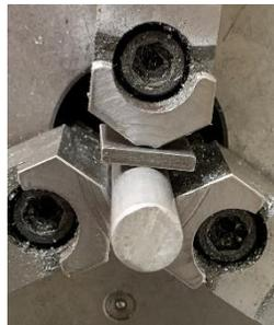
It is common practice to add a shim of precise thickness between one jaw and the stock in order to achieve the desired eccentric location. This is a nice, fast way to go if you have the correct thickness shim. If not, you must either build up this thickness with a stack of shims or machine one. Not so fast anymore.
