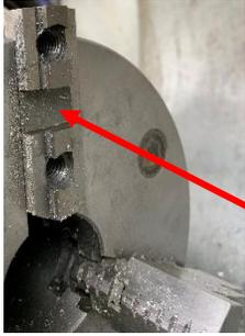
My solution depends on having a 3 jaw chuck with removable jaws that keep the jaw carrier in the chuck body.
