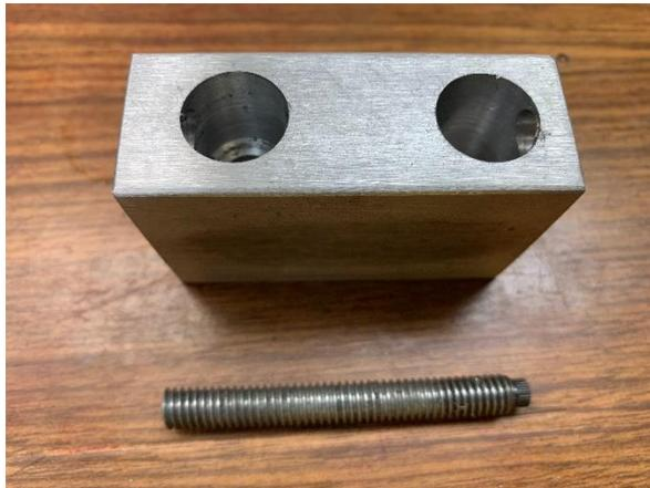
The jaw was made from aluminum and cut to be compatible with the bottom of the stock jaw.
