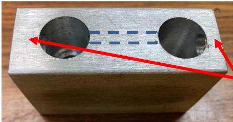
My 5/16-18 tap is not long enough to cut threads for the full length of the block. So instead, I first drilled an "F" tap hole end to end. Then I enlarged the end sections with a "P" clearance drill. This let me tap the center section shown in dashed blue lines.
