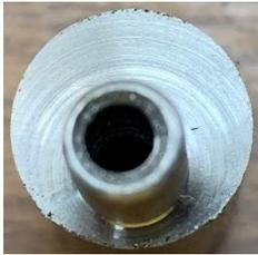
Some applications require turning an eccentric feature with high precision. For that, let me send you to Marv Klotz' outstanding eccentric calculator at [www.myvirtualnetwork.com/mklotz/#intro](http://www.myvirtualnetwork.com/mklotz/#intro) and look for the file ECCENT.ZIP. You input the desired offset and it returns the needed packing that goes between one of the jaws and the stock.
