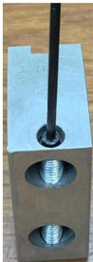
Then I use an Allen wrench to turn the threaded rod until it just kisses the stock.
