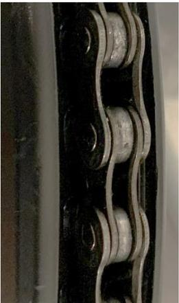
The chain is now in the gap between the sprocket and the chain guard. With the back wheel fixed, you can freely turn the crank in either direction.
