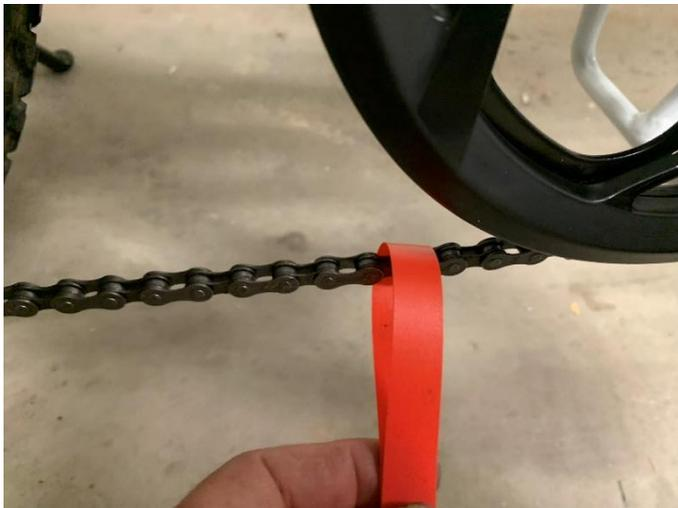
To take the bike out of neutral, wrap the tool around the chain and pull horizontally about 1/4 inch. The chain should shift back onto the front sprocket as you start to turn the crank counterclockwise. Listen for a clatter as the chain engages with the sprocket.
