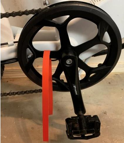
This is a potentially dangerous condition. If you jump on the bike and push down hard on a pedal, it will offer little resistance and could throw you. I remind myself that I'm in neutral by looping the tool through the sprocket spokes.
