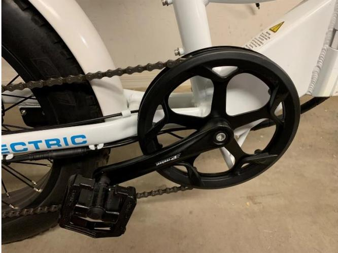
The front sprocket has a chain guard around it. The chain engages with the sprocket while being flanked by the guard.
