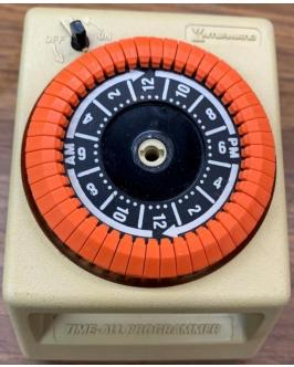
Using a thin-bladed screwdriver, I gently pried up on the center disk. Two tines on the end of the center rod grab to hold the disk in place. I broke one as I pulled off the disk, but the disk still holds well enough.
