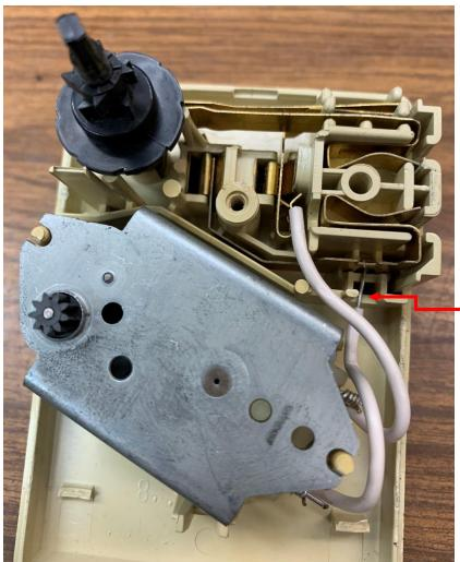
The remaining conductors are formed pieces of spring steel with a copper coating or are phosphor bronze. The only wires present are to the motor.
