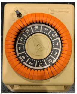
Over the years, I have accumulated many of these mechanical timers. Pull up the orange pegs to define when the output is live every 24 hours.
