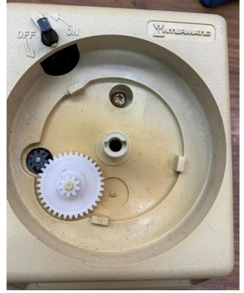
to expose the gear, which also lifts off.
