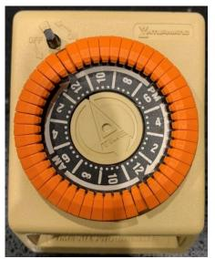
To use my new countdown timer, I turn the dial clockwise until the pointer is on one of the 12s. Then, I pull up all the orange pegs where I want the timer to run and the output to be hot. Push all pegs down where you want the timer to stop and the output zero. For example, if the pegs are pulled out from 12 to 4, I will get power for 4 hours.
