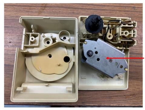
With the front cover off, you can see the motor. It rests on two pins; I will lift it off when I rewire it.
