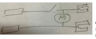
All I need to do is move the hot lead on the motor to the other side of the switch. Then, I will manually close the switch, and the motor will run until the movement of the dial opens the switch. At that time, the motor will stop running.
