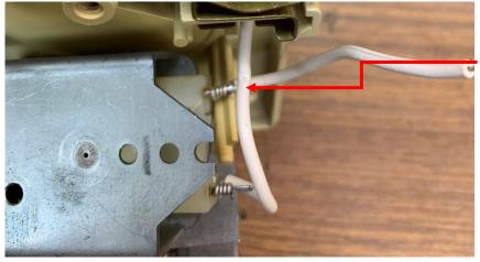
Following this wire around to the motor, you will find the end wrapped around a peg. It unwraps without using tools.
