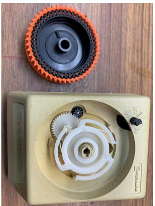
The disk with the orange fingers plus hour markings lifts off.
