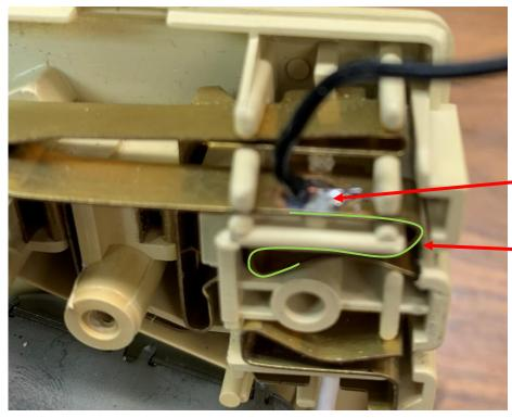
I cut off about 3 inches of insulated solid copper 24-gage wire. Next, I stripped about ¼ inch of insulation from one end and "tined2" the bare wire.
