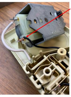
I stripped about ¾ inch of insulation from the other end of the wire and wrapped it around the pin on the motor. And finally, I soldered the wire to the pin.
