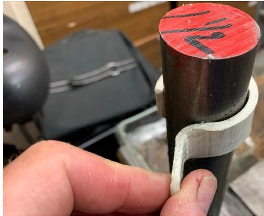
Once the plastic became soft, I squeezed it onto the mandrel and then sprayed on the water.
