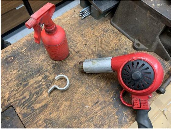
The trick is to heat the plastic up with a hot air gun until it is pliable like thick leather. Then it can be molded by hand. I use my bare hands, but if you are sensitive to heat, gloves are enough to protect you.
