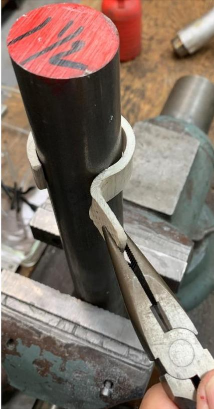
Using a piece of 1½ inch diameter round stock as my mandrel, I heated up the plastic while holding it with pliers.
