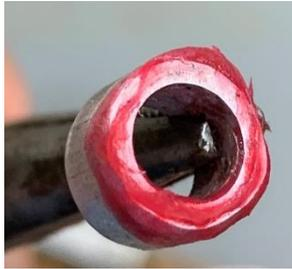
The first step is to evenly coat the lower mold with the release agent. This is accomplished by coating the end of the ring. There must be no bare spots but I don’t need to worry about having too much.
