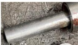
The shaft is  $\frac{1}{4}$  inch diameter rod drilled and tapped at both ends for 6-32. It is long enough to pass through the plate and upper mold and stick out the top by at least  $\frac{1}{8}$  inch. This makes it easier to place the spring on top of the upper mold.
