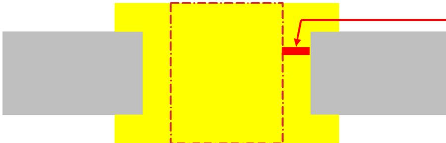
I want a grommet wall thickness of at least 0.02 inches which means the hole in the plate must be at least  $0.25 + (2 \times 0.02) = 0.29$  inches in diameter.
