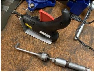
Of course, I need my hot glue gun. I also need a length of  $\frac{1}{4}$  inch diameter rod bent in an “L”. I’m holding it in my homemade pin vise because it will get rather warm.
