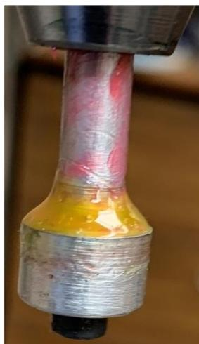
Feed hot glue into the mold by applying it in layers. The goal is to not have any voids. A quick blast from the hot air gun and I get an even cone between the top of the mold and the shaft. This cone centers the grommet in the plate's hole.
