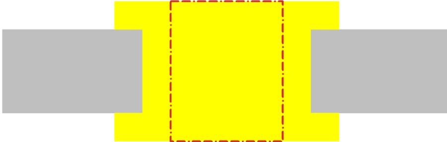
This is a cut-away side view of the grommet (yellow) molded into a plate (gray). The dashed red line is the hole through the grommet.
