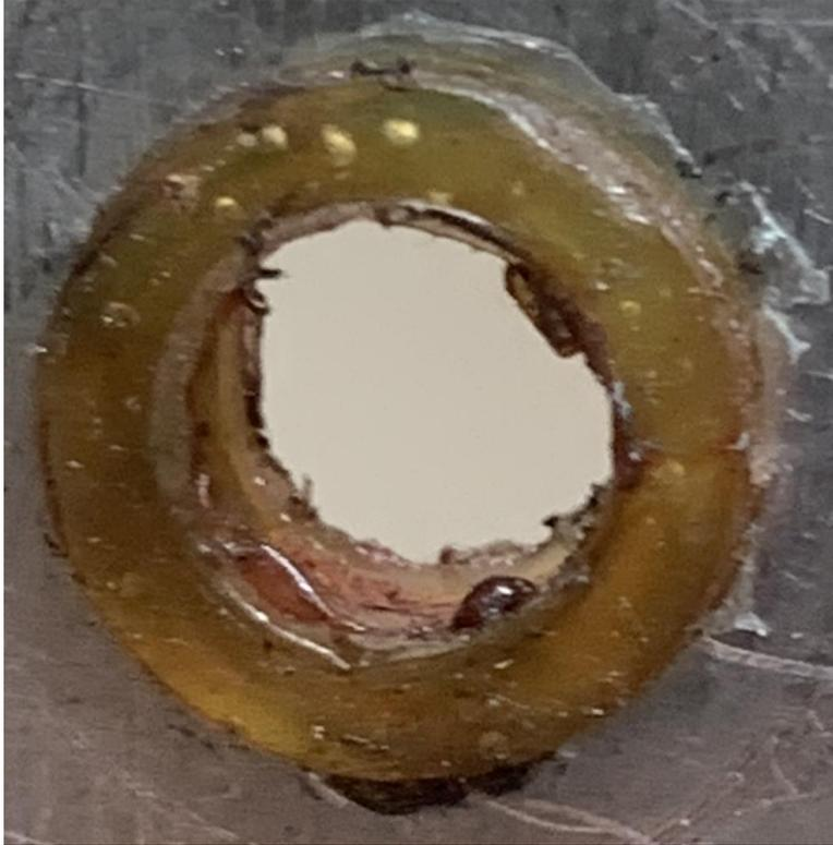
This close-up shows how the grommet fully covers the edges of the plate. The hole is ¼ inch in diameter.
