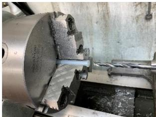
I chucked up a stick of the white hot glue in my lathe and drilled a ¼ inch hole.
