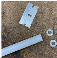
Then I used a razor to slice off two wafers about 1/16 inch thick.
