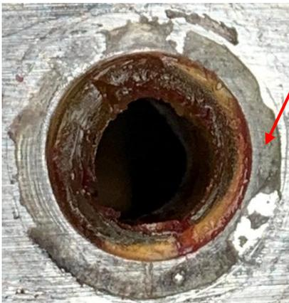
The lower mold and rod also easily slide out. It has a similar ring of flash.
