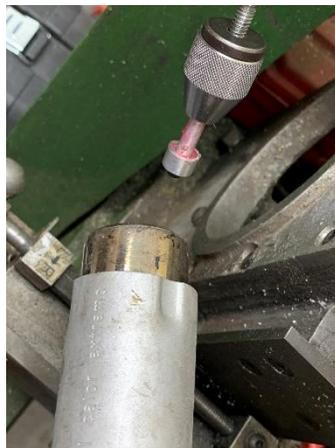
Then I use my heat gun to warm the lower mold. If in doubt about how much heat to apply, put a dab of hot glue on the mold. When it melts, it is ready.
