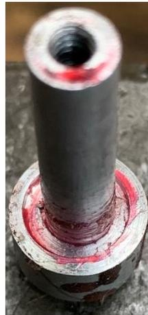
After pushing the ring down into the lower mold, I rotate it a bit. This evenly distributes the release agent into the mold plus forces it against the inside bore and the bottom.
