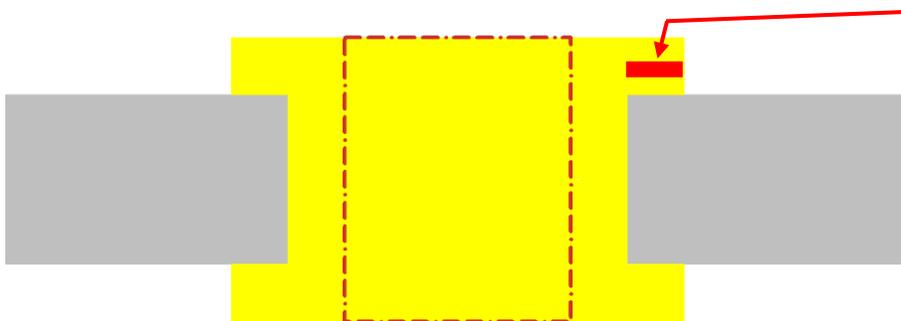
I also want the flange to have at least 0.02 inches of plate under it. This means the maximum hole size is  $0.375 - (2 \times 0.02) = 0.335$  inches. If you know the size of the hole, you can work backward to design the upper and lower molds.
