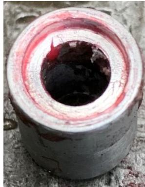
The red color of the grease makes it easy to identify any bare spots. There are none here.
