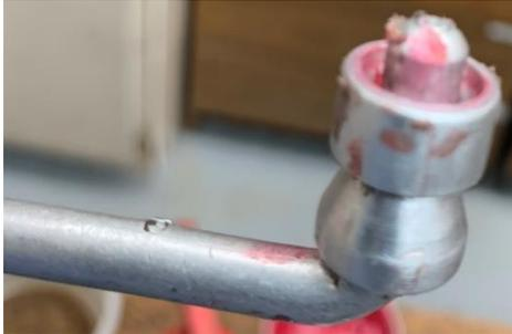
The upper mold is then placed on the rod. That fancy shape of the mold is left over from a previous project.
