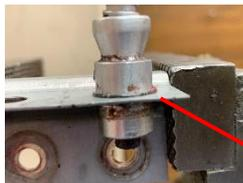
After using my heat gun, the molds move together and the wafers of hot glue enter the molds.
