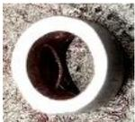
The mold release ring is a loose fit to the  $\frac{3}{8}$  inch bore and is drilled out for a sliding fit on a  $\frac{1}{4}$  inch rod.
