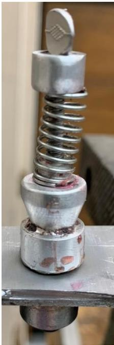
Showtime! The lower mold with rod slides up from below. The cone of glue centers it in the plate’s hole. Then the upper mold slides in from the top. Next comes the spring which is followed by the ring. And finally, I screw in the thumbscrew so gentle pressure is applied through the spring. This force must be enough to pull the lower mold up to the plate.
