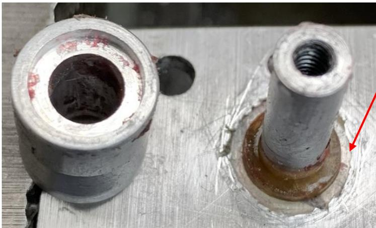
The upper mold easily lifts off to reveal the upper flange. A thin coating of flash is around it. This can be removed with a razor blade.
