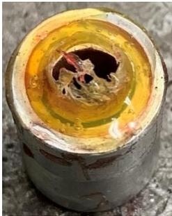
I again preheat the mold with my gun, apply hot glue into the mold, and formed a cone. After it cooled, I pulled the mold off of the rod. The bit of flash over the hole is harmless.
