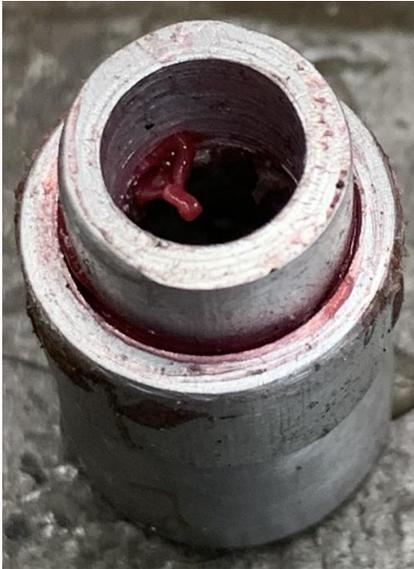
After the ring is again coated with the release agent, it is pushed down into the upper mold. The goal is the same – evenly coat the bore and bottom of the mold.
