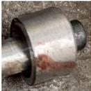
The lower mold is drilled for 6-32 clearance. The upper mold is drilled for a sliding fit on a  $\frac{1}{4}$  inch rod.
