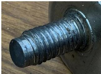
Then I spun on a nut as a guide and filed off the last 1/4 inch of thread. This made it easier to align the new nut by feel plus require fewer turns to snug it up.
