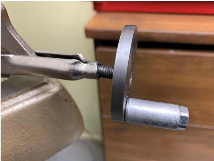
The adjustment screw was fitted with a disk of mild steel I found in my junk drawer.
