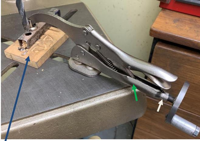
With this crank (red arrow), I can hold the end of the clamp (white arrow) and quickly turn this screw in and out.
