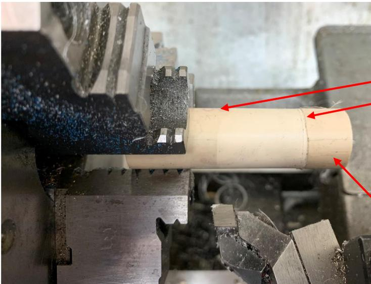
I chucked up a length of stock and cut my external taper starting about  $\frac{1}{2}$  inch from the right end.
