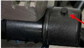
A notch was then cut axially in the internal taper part in order to pass the stud.
