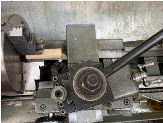
Standard practice is to adjust the compound to the desired angle and make the cut.
