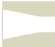
Recently I needed to cut matching tapers on my lathe. The green shape is the outline of my external taper. The tan shape is a cross section of the internal taper.
