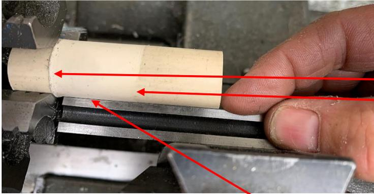
I removed the stock, flipped it end-for-end, and secured that ½ inch section in my 3 jaw chuck. This gave me a taper that was at maximum depth on the left and minimum depth on the right. In other words, this is the shape of the internal taper.
