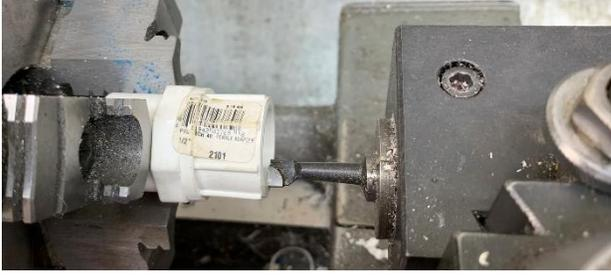
Then I changed to a small boring bar and cut the internal taper.
