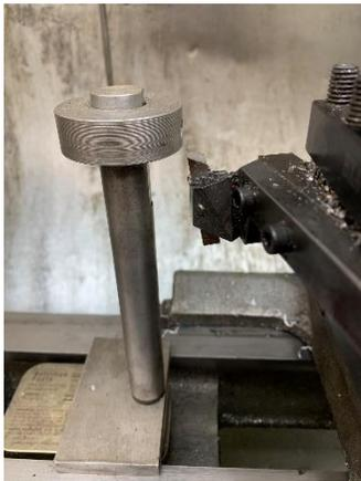
Before using the cutter, I verified that it was on the center of rotation of the chuck by using this tool. It contains a go/no go test with audible warning. See <https://rick.sparber.org/lchg.pdf> for details.
