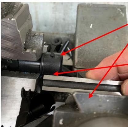
The first step was to set the external taper. The task was made far easier because I had a sample. With the Quick Change Tool Post aligned with the major axis of the compound, I used my parallel to set the compound to be parallel to the taper. Then the compound was locked so it could not rotate.
