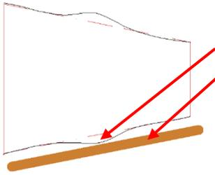
I saw that the plastic molded taper of my sample was not a straight line when compared to my parallel. It had a bump around its perimeter due to imperfections in the molding process. This meant that my best approximation was to sight the gap between sample and my parallel. By placing a strong light under this gap, it was possible to see extremely small misalignments. Trying to use a Dial Test Indicator to set the angle of the compound would not have given me the best approximation to this taper.
