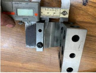
Then I move to the other end of the bar with my caliper and nudge the bar, so it is the same distance. This puts the bar parallel to the edge of the plate. I then tightened the screw.
