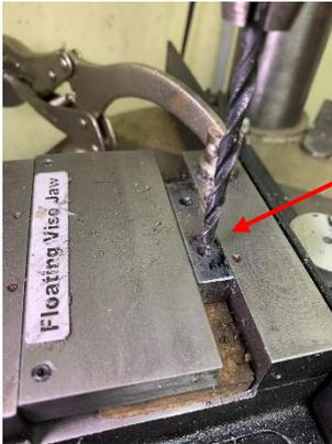
I then slide the vise along the fence with the spud installed and stopped at my scribed line.
