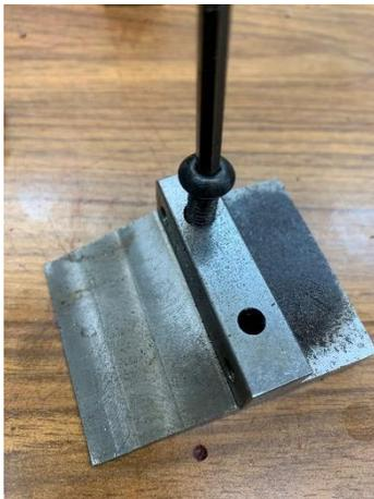
I'm running a 1/4-20 button head screw down the tapped hole until it is tight.
