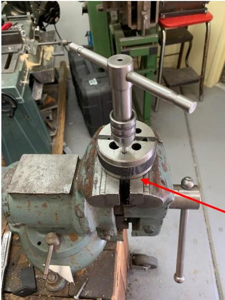
After coating the tap with cutting oil, I passed it through the bench block and into the bar. This keeps the tap vertical as I cut the threads.
