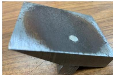
After sawing the excess screw off on my bandsaw, I sanded it flat on my belt sander.
