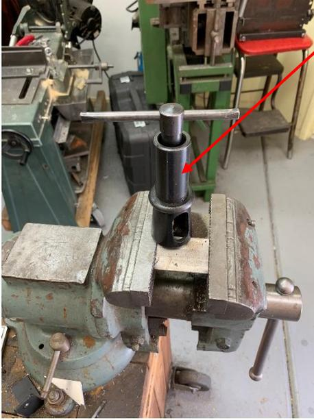
My 1/4-20 tap was fitted into this tap handle with built-in base. After aligning the top of the plate with the top of the vise jaws using my magnet trick, I tapped this first hole. Then I deburred it with my brace-and-bit.
