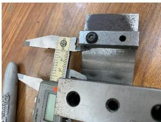
With my 1-2-3 block against the edge of the plate, I lock my caliper to the distance between the face of the 1-2-3 block and the bar.
