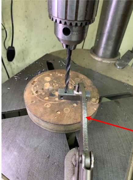
Then I used my #F drill to open out the #4 hole in the bar. I am only enlarging the hole that I used to locate the hole in the plate.
