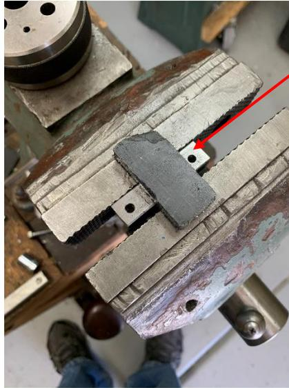
I stuck the magnet to the bar and placed it between the vise jaws. This ensures that the top of the bar is flush with the top of the vise jaw. After tightening, I removed the magnet.
