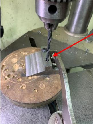
Moving back to my drill press, I lowered the #4 drill through this second hole. Then I clamped the plate down.
