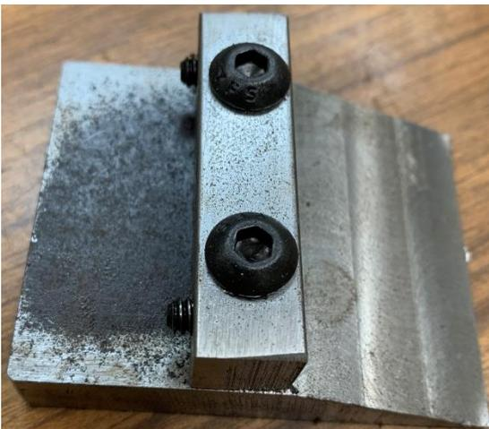
I tapped the second hole and deburred it. Then I ran the second button head screw, sawed off the end, and sanded it flat. And finally, I ran two set screws in those horizontal holes.
