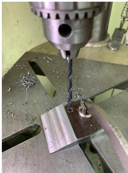
After clamping the plate down, I removed the bar, used my spotting drill, and my #4 to go through the plate.
