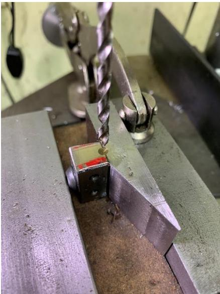
I fitted the block on the plate and placed it in my drill press vise on its side. Then I used my spotting drill to cut a cone at the joint between the block and the plate.
