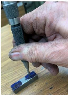
I used my spring-loaded punch to mark the crossed lines on one end.
