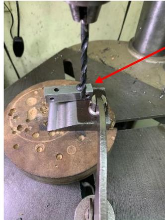
Next, I loosened the screw, swung the bar away, and tightened the screw. I do not want that bar swinging into the drill bit as I cut my second hole in the plate.
