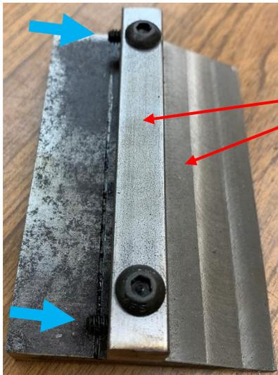
The part I am fabricating is unimportant. I want to focus on the steps I used to drill and tap the holes that secure the bar to the plate using close-fitting screws.
