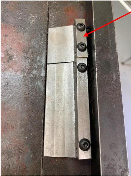
I installed another bar to a plate that was half as wide. The button head screws are again  $\frac{1}{2}$ -inch from the ends, and the 10-32 set screws are  $\frac{1}{4}$ -inch from the ends.
