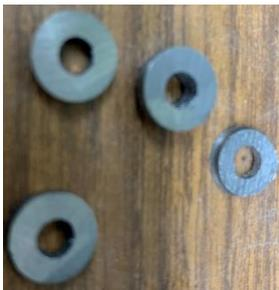
Here is a sample of #6 washers of various thicknesses. All are 3/8 inches in diameter.
