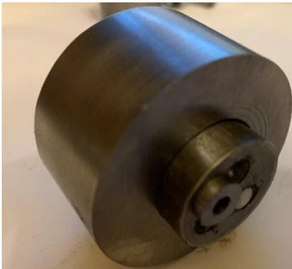
With the set screw loose, I raise the platform until it is proud of the guide. Using my finger, I wipe the surface clean. Those magnets certainly attract swarf. I then place the deburred face of the rough washer against the platform.
