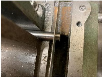
When I want to make a washer or spacer of a given thickness, I first deburr the end on my belt sander. Then I saw off a piece about 0.05-inches longer. This is my rough washer.
