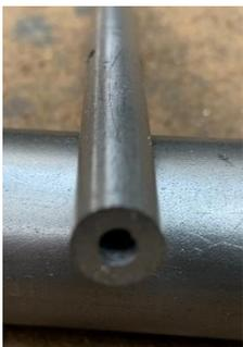
I start by selecting steel round stock with the desired Outside Diameter. Then, using my lathe and the proper drill bit, I drill down an inch or two. Take it slow and pull the drill out often to remove swarf. Use plenty of cutting fluid. This will keep the drill going straight.
