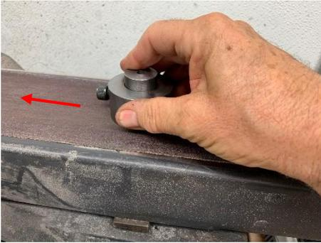
Position the fixture in your hand so the set screw is pointing in the direction of the belt's motion (red arrow). This prevents the washer from jumping to the other side of the bore.
