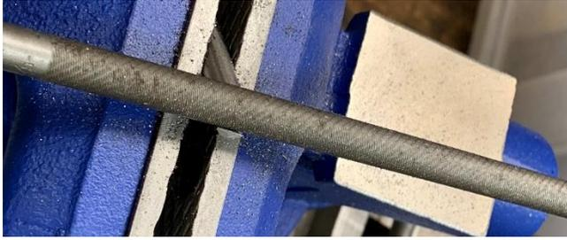
Using a fine file  $\frac{1}{4}$  inch in diameter, I cleaned up the cut.
