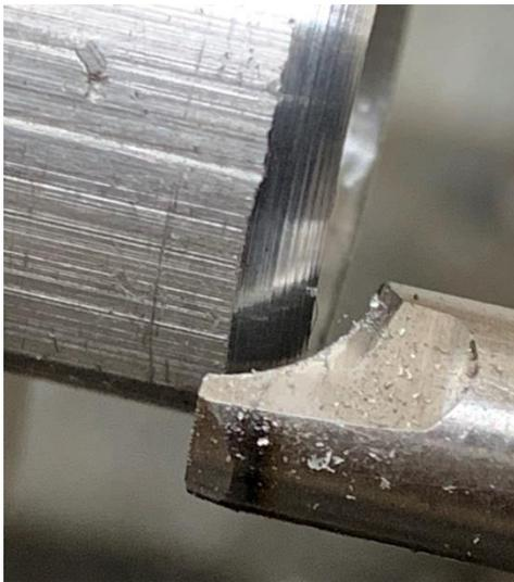
That got me thinking about making my own corner radius tool. The radius here is about  $\frac{1}{4}$  inch. The cutter is made from water hardened rod but since I’m cutting aluminum, I didn’t harden it.
