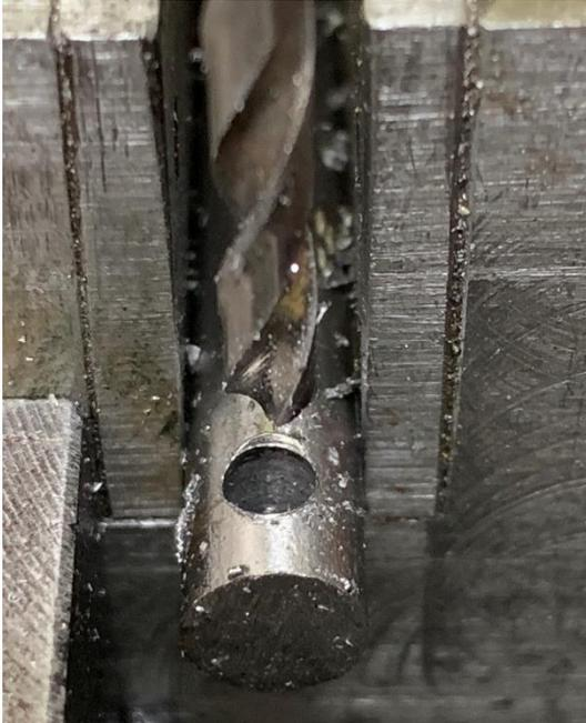
Next, I cross drilled with a sharp 1/8 inch drill. Used plenty of CoolTool.
