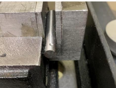
After sawing off a 2-inch piece of rod, I clamped it into my small vise which was then clamped into my drill press vise. I chucked up a piece of  $\frac{1}{4}$  inch diameter rod and lowered it into the gap between the vise jaws. This gave me my center. Using plenty of CoolTool, I drilled this divot with my spotting drill.
