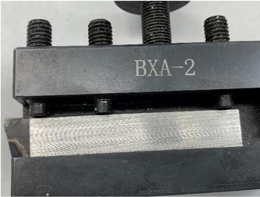
The beveled aluminum bar goes in next with the bevel facing out. As the screws are tightened, the bar is pushed both down and deeper into the slot. This securely clamps the blade.
