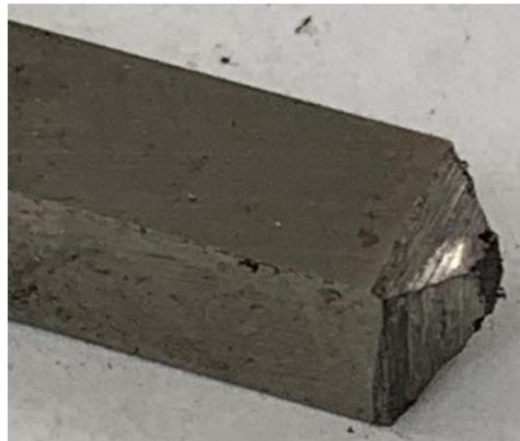
This may not look like a tragedy to you, but it crushed me. I had spent a very long time grinding this slug of 1/4" by 1/4" High Speed Steel to have a nice 0.05" wide cutter on the end. In an instant, it was an ugly stub.
