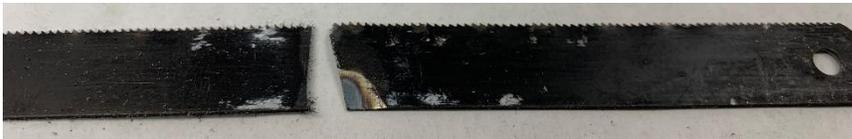
Then lop off a length of hacksaw blade<sup>4</sup> and put some relief on the end. The piece on the right will be my grooving tool.
