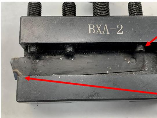
Then I placed the piece of hacksaw blade into my BX A tool holder and tilted it so the back top edge touches the top of the side slot
