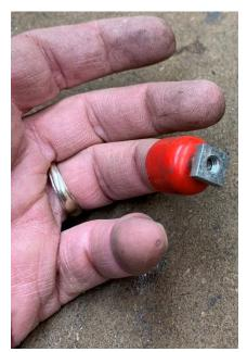
The cap fits snuggly on most of my fingers and securely holds the nut. The head of the 2-56 screw centers the 10-24 nut.
