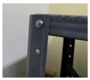
I needed to add a 10-24 nut and bolt to the corner of a shelf unit. It should be easy.
