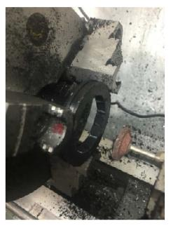
With the lathe running at around 100 RPM and the grinding wheel turning at 35,000 RPM, I took 0.01 inches per pass. In just a few minutes I was done with the ring.
