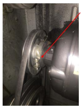
After over 25 years of service, one of the rubber support rings that holds the motor in my Atlas/Craftsman lathe failed. A search of the web found nothing that perfectly fit. The closest I could get had the correct outside diameter but the wrong inside diameter. This is how I machined two of these rings so they would fit.
