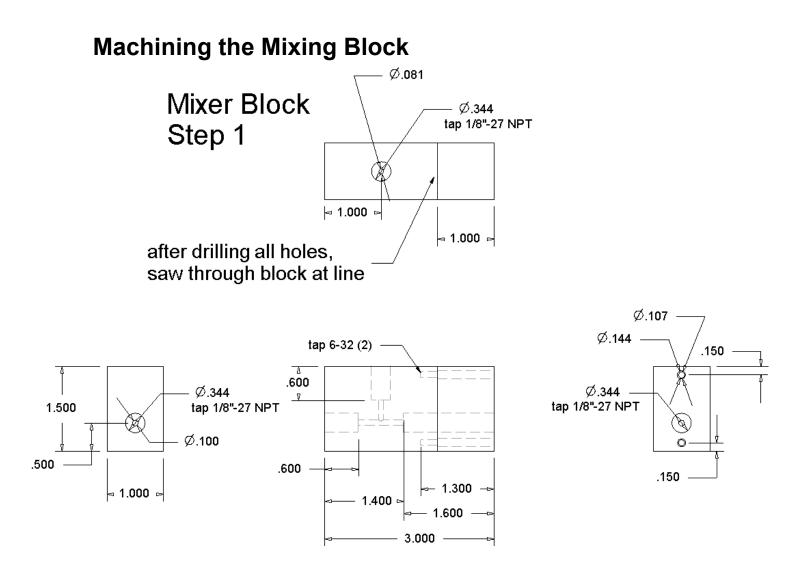
In step 1, I squared up a block of 6061 aluminum. Then I drilled the holes shown here. Although not shown in the drawing, I counterbored the 6-32 holes so the screw heads are recessed.
