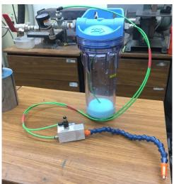
I built a modified version of the Minimum Quantity Liquid (MQL) Coolant System designed by Brian Lamb. It is running a 5% solution of Tri-Cool<sup>TM</sup> mixed with water and is propelled by a stream of air at about 10 PSI.
