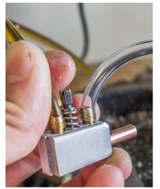
Jason used barbed hose fittings, clear plastic tubing, and a homemade needle valve. On the left end of the mixing block is a dovetail. This permits him to mount the mixing block on a DTI support.
