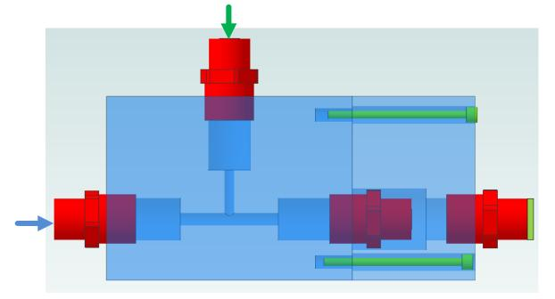
With the block translucent, you can see the internal passageways. Air flows in from the left (blue arrow), liquid from the top (green arrow). They mix at the upside-down T and flow out the coupler hidden inside the block. The coupler shown on the far right (with the green rectangle) is part of the Loc-Line assembly.
