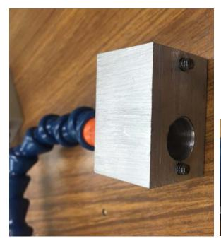
I install the two 6-32 by 1.25 inch long SHCS bolts in the smaller block. Then I screwed in the Loc-Line. I turned the hex on the Loc-Line until the flat is parallel to the bottom face of the block. This will give you maximum access to the lower screw head.
