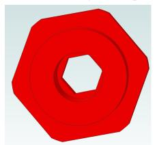
If you look down the bore of these couplers, you will see a section that grabs the tube. This section both locks the tube in place and forms an air tight seal. The adjacent section is a smaller diameter and has a hexagonal hole. As you push in the tube, this smaller diameter prevents further penetration.
