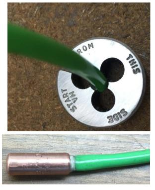
Next I coiled up a handful of tubing and hand feed a 10-24 nut onto the end for about  $\frac{1}{4}$  inch. This formed a shallow thread and made it easier to turn the 10-24 die onto the end. Only need about  $\frac{1}{4}$  inch of thread.
