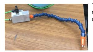
This mixture of coolant and air feeds through the blue ¼ inch Loc-Line<sup>™</sup> and out the nozzle.
