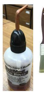
A bottle of cutting fluid and a brush can be used to lubricate a cutter and remove chips. This prevents the chips from being re-cut which can cause a bad finish or even break the cutter. It takes constant attention but does work. If manually milling, this approach isn't so bad. You have to be there anyway.
