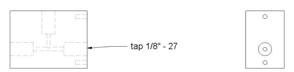
In step 2, I tapped the outlet hole in the larger block. The I trial fit a coupler but this time left it in.
