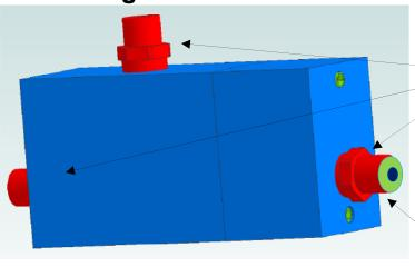
This rendering of the mixing block shows the liquid inlet, air inlet, and output.
