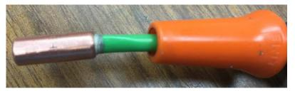
Note that the Loc-Line only provides mechanical support. The coolant/air mixture flows through a tube inside the Loc-Line.
