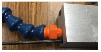
After trimming off the end of the tube, I inserted it back into the coupler. I Slid the blocks together and tighten the two 6-32 SHCS bolts.
