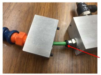
I pushed the tube all the way into the coupler. Then I slid the smaller block down until it contacts the larger block. The MIG tip rose out of the nozzle a bit. I measured from the end of the nozzle to the end of the MIG tip and subtracted 0.2 inches. This is how much I needed to remove from the tube at the coupler end. I released the tube from the coupler by pushing in on the ring while pulling the tube out.
