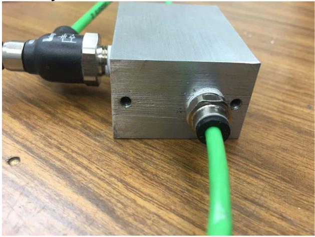
Using Teflon<sup>TM</sup> tape<sup>4</sup> on all threads, I tightly screwed in the needle valve, air inlet, and mixture outlet couplers into the larger block.
