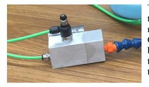
The mixing block has two inputs. On the top is the liquid line. It feeds into a needle valve making it easy to control the flow of coolant. On the side is the air line. Holes drilled in the block channel the air past the liquid. Due to the Bernoulli's principle, coolant is drawn into the air stream.
