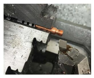
I put the 0.035 MIG tip in my lathe and face the end to remove the external threads. Then I used a #25 drill and went in about <sup>3</sup>/<sub>4</sub> of the length of the tip. Using a 10-24 tap, I cut threads as deep as possible.
