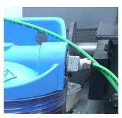
The tube passes through an air tight fitting and out the right side.
