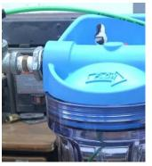
The rest of the air feeds into the coolant tank. This tank is just a whole house water filter housing.
