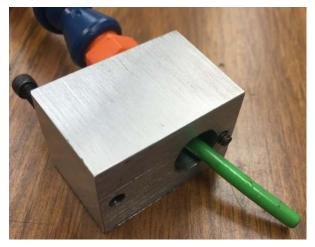
Next I cut the tube off at the block end with about 1 inch exposed.
