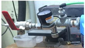
Compressed air at about 10 PSI is fed in from the left via a ball valve<sup>2</sup>. Most of this air flows out the T and into the green line.
