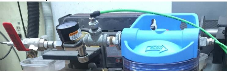
I used wrought iron piping except where my junk drawer provided brass. I figured that the coolant does not rust the machine so it should not rust my pipes. Don't forget to use Teflon tape at all joints.
