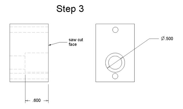
Next I drilled the recess in the smaller block to provide room for the hidden coupler. I trial fit the blocks together to be sure the smaller block does not hang up on the hidden coupler.
