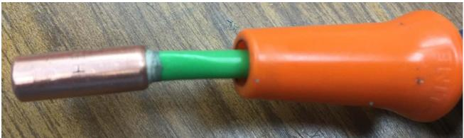
I needed to remove a small amount of plastic from the inside of the Loc-Line nozzle so the MIG tip can freely slide inside. A tapered reamer fed from the wide end of the nozzle did the job. Very little plastic must be removed.
