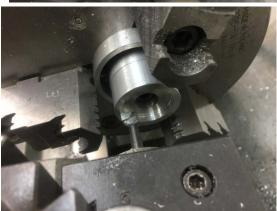
I then use a boring bar to lightly face the end. Since this counterbore is so large, there isn't much to remove. Yet I do get the maximum diameter contact area for the part to be machined.
