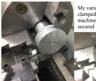
My variation is to have an aluminum cylinder clamped to the face of the spindle. The part to be machined contacts this cylinder and is then secured with the jaws of the chuck.
