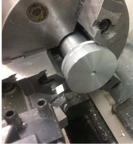
I then take my facing cut on the part. Back out the jaws, wipe the surface clean, flip it over, and use the same procedure to insure the part is in full contact with the face of the small cylinder. Then I take the second facing cut.
