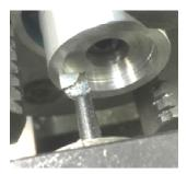
This cut makes the stop essentially a "soft stop" since it is in the same family as "soft jaws<sup>2</sup>" which are machined in place for maximum accuracy.
