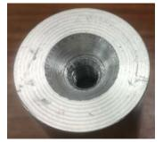
The back end of the larger cylinder was drilled and tapped to accept the draw bar but also has a generous tapered opening. The taper makes it easier for me to slide the draw bar into the threaded hole.
