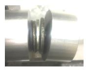
Having the small cylinder as a separate part provides an easy way to adjust its position. I can stack up washers between the cylinders
