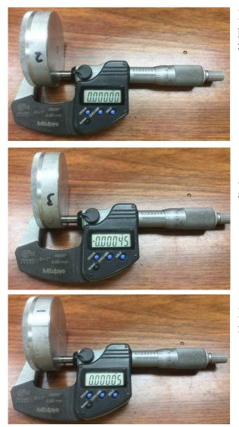
I marked three location around the test piece about 120° apart. My mic was zeroed at location 1.
