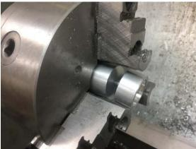
With the large cylinder locked in place, I can now tighten down the  $\frac{1}{4}$ -20 screw.
