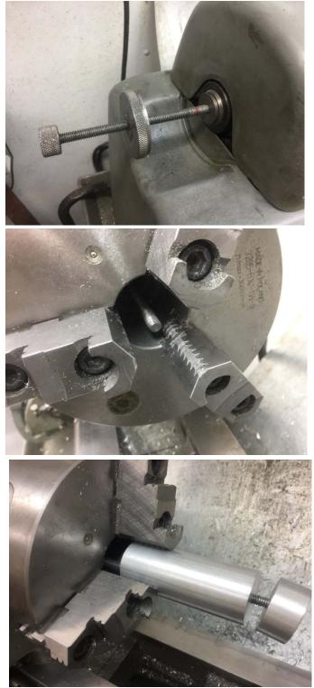
First I carefully clean the bore of the 3 jaw chuck and the end of the spindle. No swarf should be in this area.
