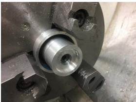
Next I back out the jaws and insert my safety ring. It insures the jaws are a safe distance from the end of my small cylinder plus puts tension on the jaws. With no tension, there is a chance the chuck scroll could spin and send jaws flying away as it turns at high speed.
