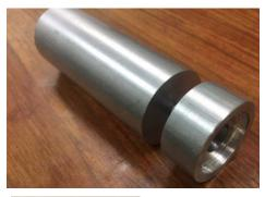
You can see that my cylinder is actually made from two pieces. The forward end of the larger cylinder has been machined flat. Then I drilled and tapped it <sup>1</sup>/<sub>4</sub>-20. The smaller cylinder has a flat rear face.
