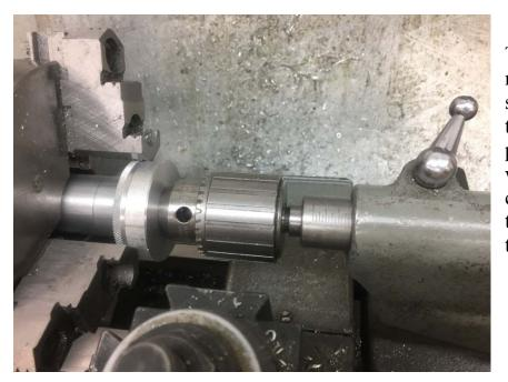
Time to install the part to be machined. With all contact surfaces clean, I use the tailstock to apply pressure to the part so it will be in full contact with the face of the small cylinder. Then the jaws are tightened. Slide back the tailstock.
