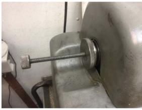
Next I spin the take up nut to draw in the cylinder. When tight, the bottom of the cylinder locks onto the end of the spindle.
