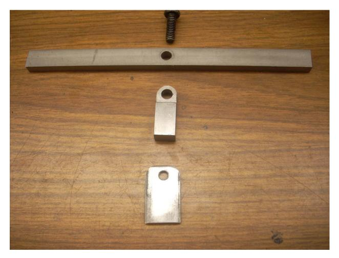
Not much to it. The rounded bar in the center gives a rough alignment of the fence to the T-slot but I still need to use my machinist square to get it right.
