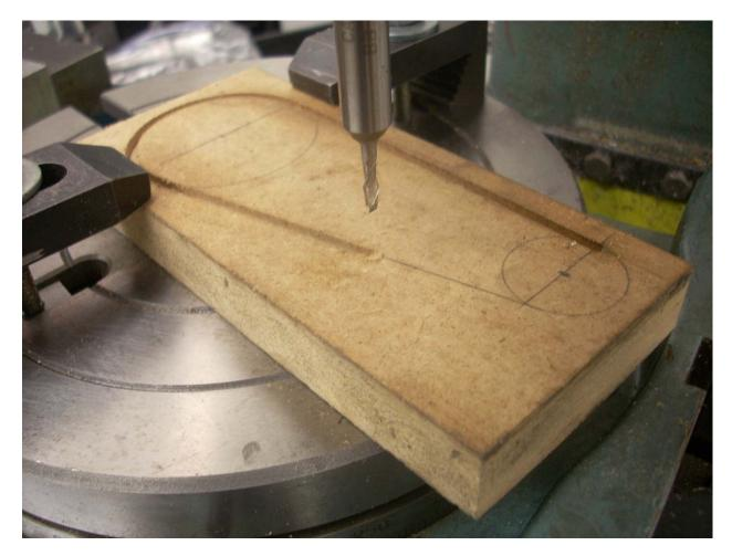
You may wonder why I stopped half way along the line. Well, I got caught in a lesson that keeps being repeated because I haven't learned it yet. I forgot to run the cutter over the full path before starting. My mill table is all the way to the left so the cut ends here. Time for plan "B".
