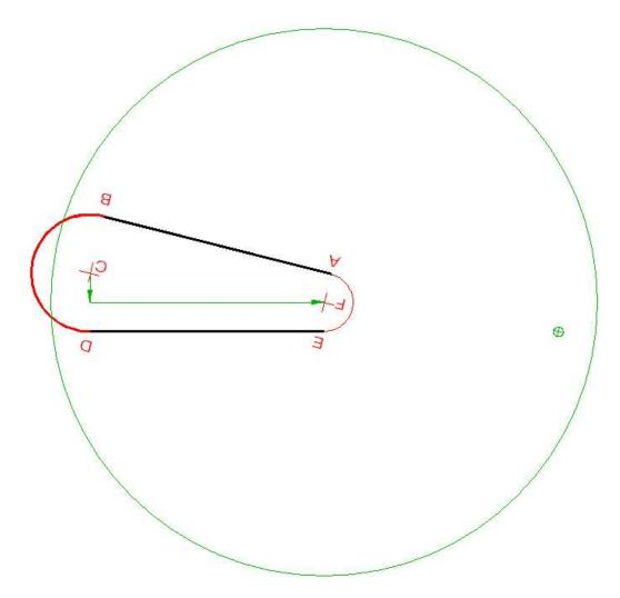
We have moved the center of rotation down and to the right which means that we have moved the part up and to the left.
