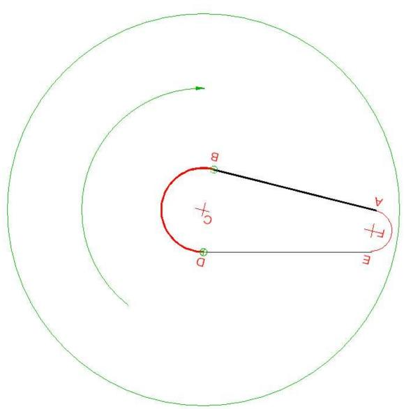
By cranking the RT 194.2°, we trace the arc and end up at point D. Note that the cutter went from point B to point D because the RT turned clockwise. It may seem strange but remember that the cutter really does not move, the part moves.
