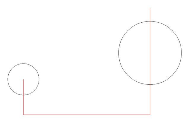
The small end has a radius of 0.500" and the large end has a radius of 1.000". They are separated horizontally by a center to center distance<sup>2</sup> of 4.000". I started by drawing a 1.000" circle on the left. A line was then drawn vertically from the center of the circle down a short distance. I then drew a 4.000" line horizontally.
