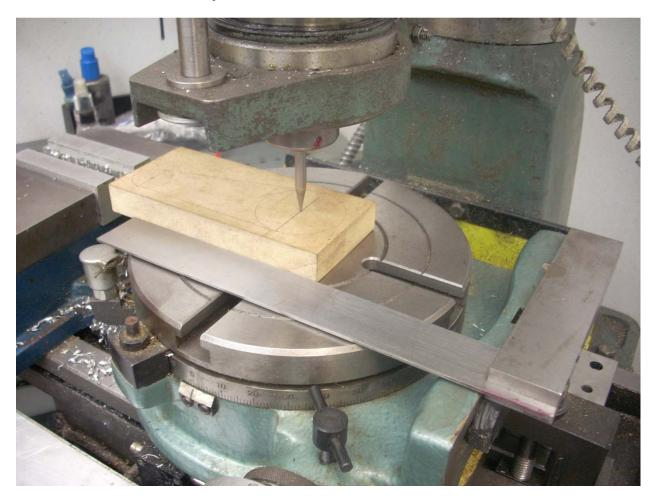
I'm using a spud mounted in a collet to hold the block of MDF while my machinist square aligns the edge. Recall that I want the center of the large arc to be aligned with my center of rotation. After clamping down the block, I mounted the end mill.
