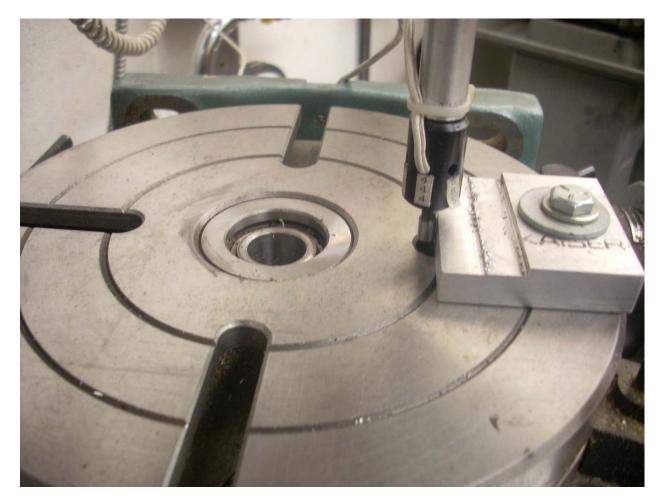
First I will align the center of rotation along the Y axis. I run the EEF, set with no tool offset, up to the block and set zero.
