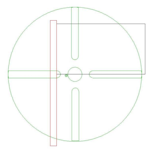
By moving the mill table in the positive Y direction, the spindle mounted rod is pushing the plate in the negative Y direction along the fence. As with the X direction, I can use the Y axis indictor to tell me how far I have moved the plate.
