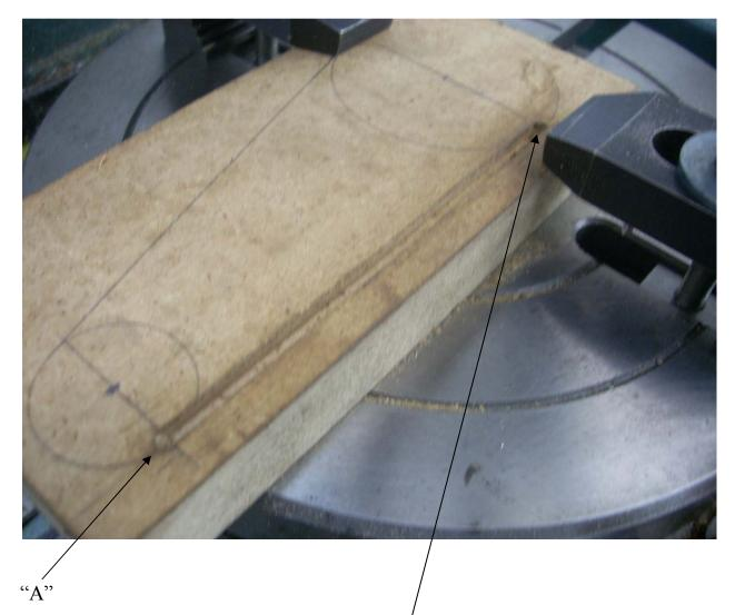
The X axis feed is driven until I get to point "B".
