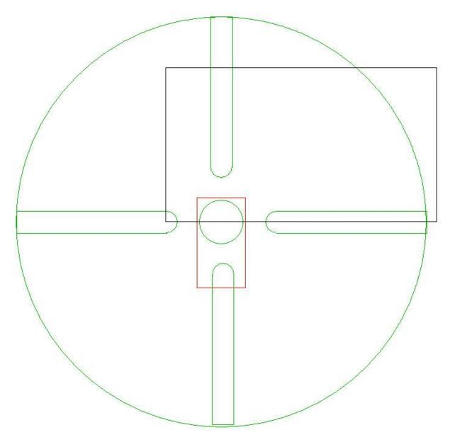
The clamp has been reapplied and the fence removed. My plate has been reposition on the RT using a fence, a clamp, a spindle mounted rod, and the accuracy of the mill table's XY positioning function. This process is a lot more bother than just using a compound mounted to the top of the RT but has the advantage of very low cost and low height. Given how many times I expect to need this function, I will gladly put up with the extra steps.
