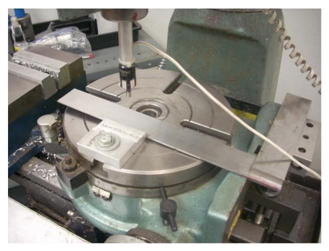
I will use an Electronic Edge Finder (EEF) and a block of metal clamped to the RT. The RT is set to 0° and the crank gear has been disengaged for now. I'm using my machinist square to get the block parallel to the X axis.
