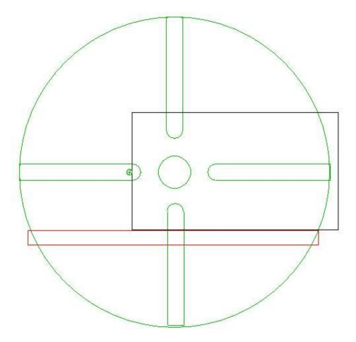
By moving the mill table to the left, my spindle mounted rod pushes the plate to the right. The fence insures that no motion along the Y axis will take place. Since no cutting is going on here, a light touch on the plate keeps it in contact with both the rod and fence. I know exactly how much the plate has moved because I can read it off of my mill table's X axis position indicator.
