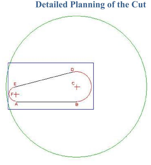
The block to be cut, shown in blue, is set up on the RT so line A-B is parallel to the mill's X axis and point C is at the center of rotation of the RT. The (0,0) point of the mill table is set up at the center of rotation of the RT.
