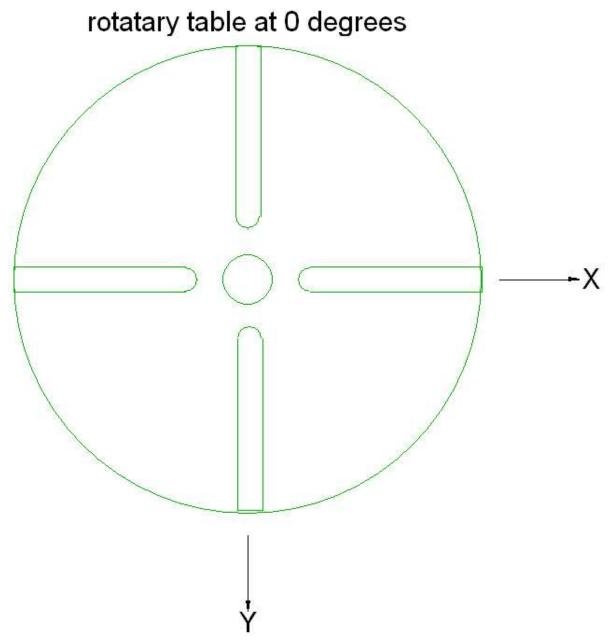
My RT is set at  $0^{\circ}$ . The center of rotation is aligned with the center of rotation of the mill's spindle. This puts my (0,0) point at the center of the RT. Note that I choose to define my positive X direction to the right and my positive Y direction to the front as the table is viewed from the top.
