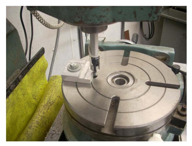
The RT is spun 180°. Then I move the Y axis until my EEF again contacts the block. Half the distance traveled is my Y = 0. The procedure is repeated for the X axis. I now have (0,0) set at the center of rotation of the RT. The crank drive is reengaged.
