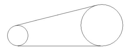
I now have each tangent 4.000" long and the center to center distance is 4.031". The lower tangent is parallel with the X axis.
