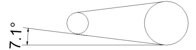
Using my CAD's measurement capabilities, I can easily find how much to rotate the figure so the bottom tangent will be horizontal. I then use my rotate tool to turn it counterclockwise by 7.1°.
