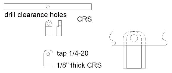
The dimensions of the various parts must come from your RT. The assembly is held together with a socket head <sup>1</sup>/<sub>4</sub>-20 screw. No need to tighten a lot since the goal here is just to prevent the fence from moving as we reposition the plate. The rounded part with the cut out was initially supposed to give me alignment to the T slot but it is too sloppy. You may wish to just make the bar and tapped part that engages the T slot.
