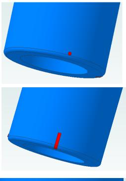
Do you fish around for the locator pin every time you insert an R8 into the spindle? Use your hand held electric drill to cut a small, shallow hole in the perimeter of the spindle right over the R8 slot. It could be 0.1" in diameter and 0.05" deep. Fill it with red nail polish and then strike off.
