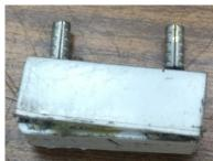
My version of the magnetic clip uses two ¼" x ¼" x ¼" neodymium magnets, two spade clips, and a few squirts of heat glue. Bits of plastic hold the clips together.
