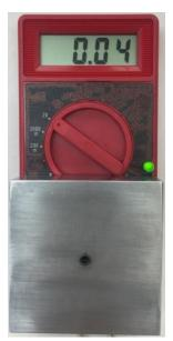
**One time only**, connect the magnetic clip to the table of the mill or ways of the lathe. Select the meter scale that displays a number rather than "1 " which means overload. Remember this number which may be positive or negative. It is your *minimum reading*.
