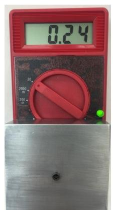
The battery enclosure is made from 1/8" X 1" X 2" aluminum channel. The top and bottom were cut on my bandsaw and then trimmed to fit on my belt sander.
