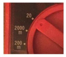
It is possible to change the voltmeter to a more sensitive range. How sensitive you can go depends on the voltage read when  $R_x$  is zero. This voltage is called output offset. My copy of the circuit shows an output offset of about -6 mV. This means an  $R_x$  of zero should give me -6 mV. An  $R_x$  of 2 ohms reads approximately 2000 mV. I can see a change in  $R_x$  of 0.001 ohms (1 milliohm). So far, I have not found a need to be this sensitive on my mill or lathe.
