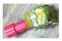
Hindsight: remove the plastic sleeve and solder the wires to the clips now. Doing it later causes the heat glue to loosen.
