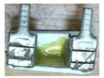
After making two of these subassemblies, I heat glued them to strips of plastic. The plastic on two sides gives the assembly strength while insulating the parts.
