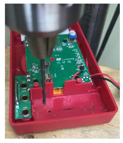
First I drilled 4-40 tap holes along the centerline of the battery compartment about <sup>1</sup>/<sub>4</sub>" from each end.
